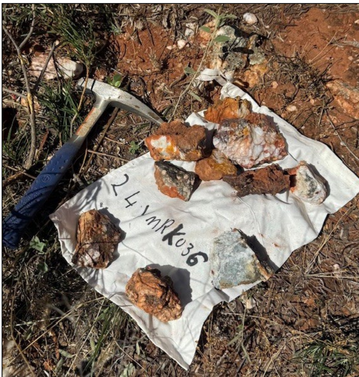
Photo 2: – Samples from Banjo's Camp target area. The Competent Person confirms that this photograph is of a rock chip sample (24YMRK036) that was laboratory assayed at 5.3 g/t Au. Refer JORC tables enclosed in this announcement for further detail.
