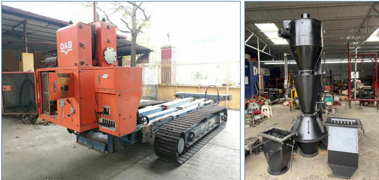
Figure 7: Track-mounted carrier for the compressor and the RC sample system
