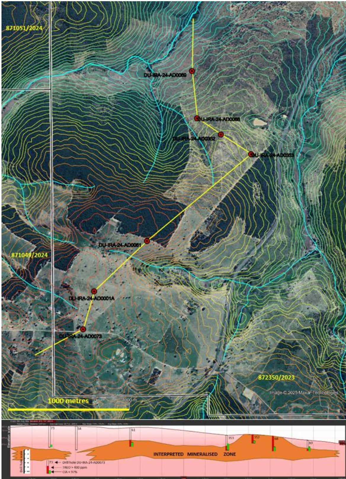
Figure 2. Drill section where drillholes intersect the top portion of the saprolite zone. The saprolite zone is the zone where most of the REE mineralization is expected to be located. TREO intersections greater than 400 ppm in red and CIA less than 97% in green.
