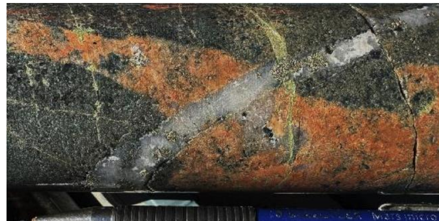
Aplite/microgranodiorite dykelet, cut by quartz+carbonate + pyrite vein, cut by epidote stringers and fractures (442.1m)
