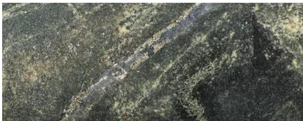
Quartz+pyrite+molybdenite vein in microdiorite / hornfels. 389m.
