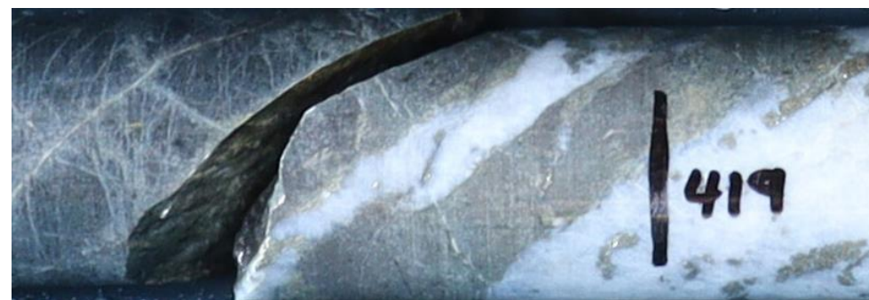
Sandstone/Andesite. Moderate pervasive chlorite, weak-moderate patchy sericite+magnetite assemblage, cut by quartz+carbonate+pyrite± calcite veins & rare aplite dyke 410-421m, with 1m@ 0.215g/t Au from 418m
