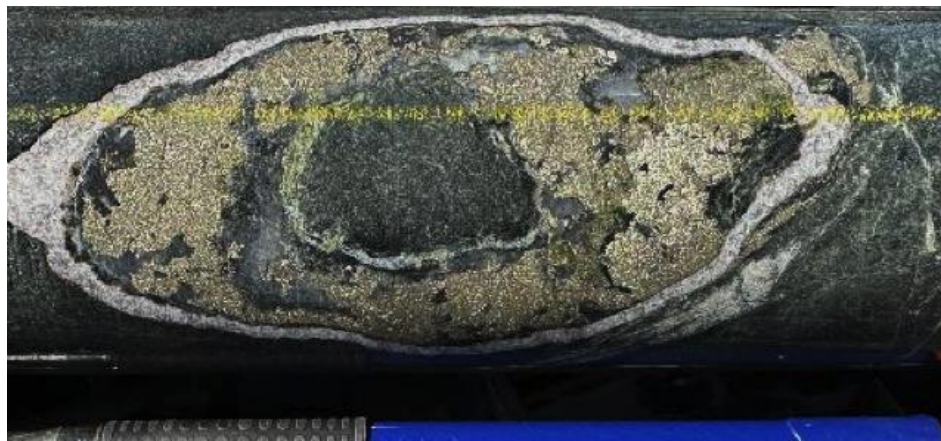
Pyrite+chalcopyrite+calcite vein. Subparallel to the core axis. 432.5m
