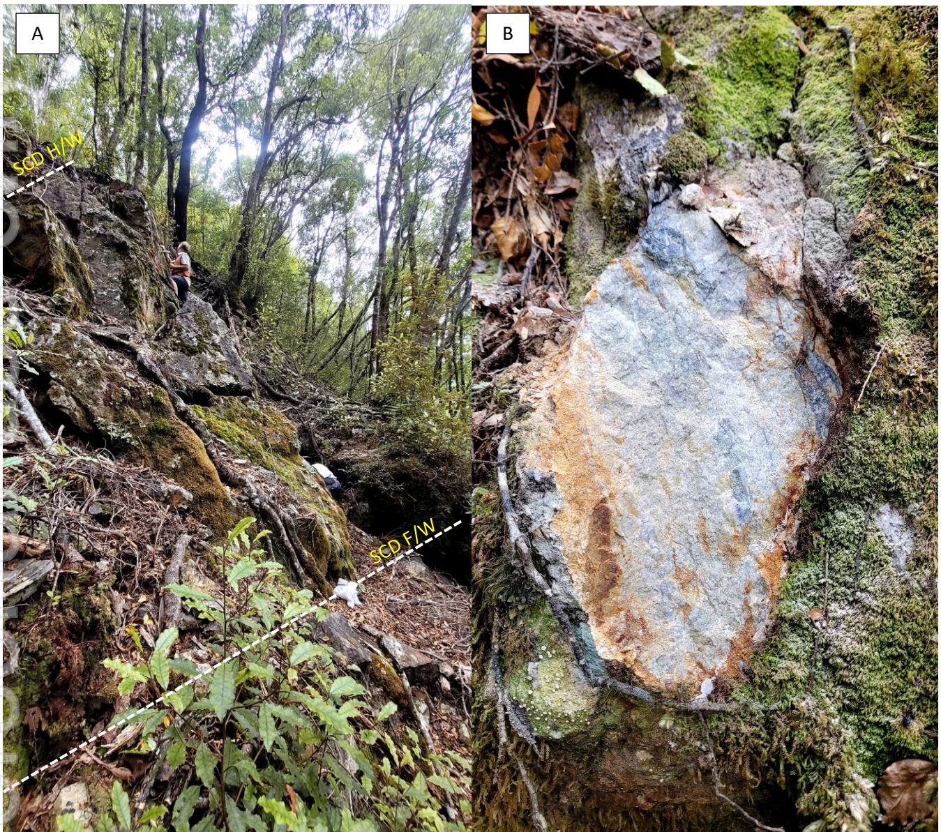
Figure 6. A. Outcrop of the SCD in the A2 Anticline at Doyles showing the hangingwall (H/W) and footwall (F/W). B. SCD footwall showing highly silicified and altered granite with arsenopyrite veinlets shown by dark grey. Rock chip assays obtained from this area have ranged from 1.0 to 9.6 g/t Au (refer table 2)
