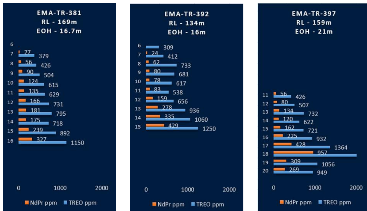
Figure 6 – Drill-hole profiles showing typical ionic REE enrichment zone with high NdPr grades close to the fresh rock interface.
