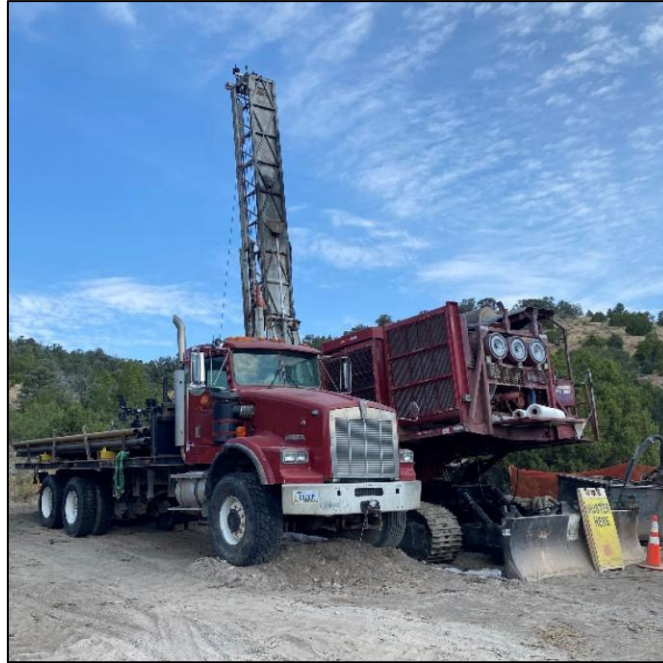
Figure 3: Alford Drilling MPD 1500 drill rig with support truck
