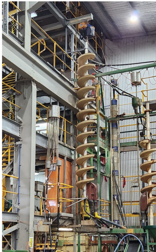
Figure 5 - Full scale spirals used in piloting.
