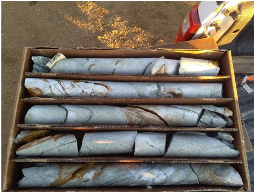
Core from GDD02 from 178 m to 181m downhole which assays 40 g/t Gallium
