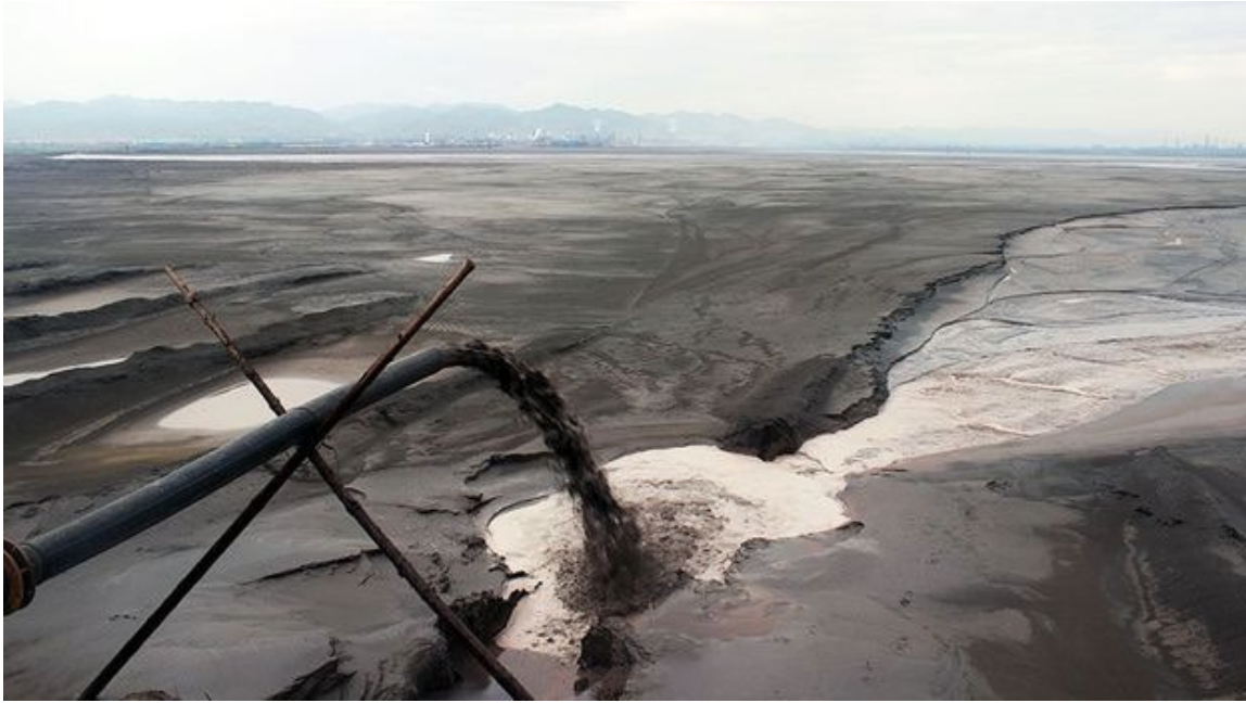
Figure 1: Tailings generated from conventional rare earth production at Bayan Obo mine, Inner Mongolia, PRC.
