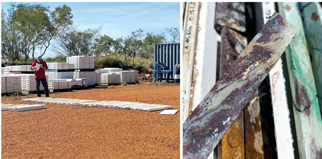
Figure 6 – COB personnel inspecting core at the Halls Creek core storage facility (Left). High-grade oxide-supergene copper mineralisation intersected by AORD004 comprising 16.6m at 10.2% Cu, 0.46% Pb, 1.03% Zn & 316g/t Ag from 130m (core pictured at approximately 137m)
