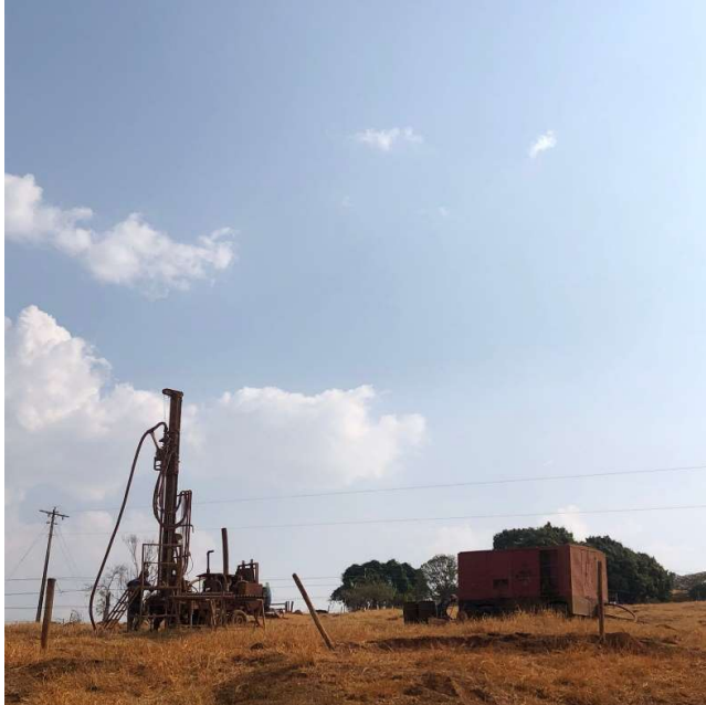
Figure 1: Reverse circulation drill rig at CODA North.
