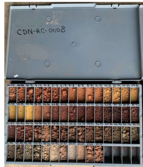
Figure 4: CDN-RC-0008 drill cuttings which has been reported as having 31 m intercept @11.2% TiO 2 including 10 m intercept @14.8% TiO 2
