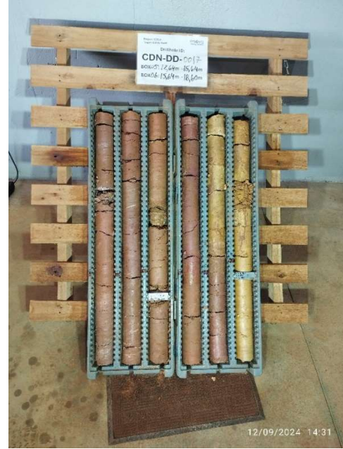
Figure 2: CDN-DD-0017 drill core which has been reported as having 16.4 m intercept @13.1% TiO 2 including 5 m intercept @16.3% TiO 2
