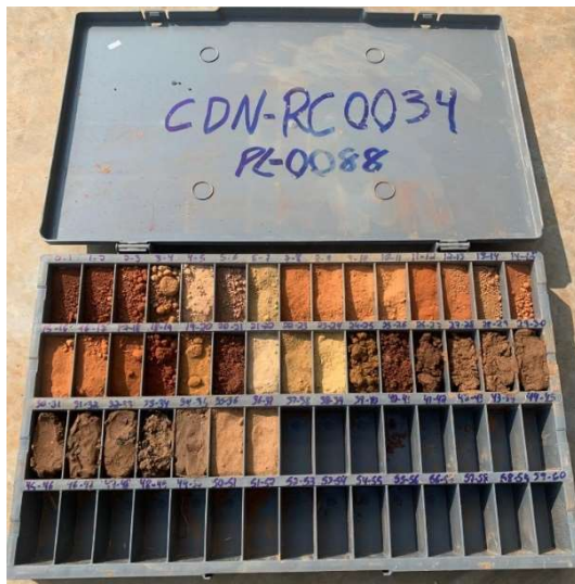
Figure 3: CDN-RC-0034 drill cuttings which has been reported as having 34 m intercept @10.0% TiO 2 including 9 m intercept @17% TiO 2
