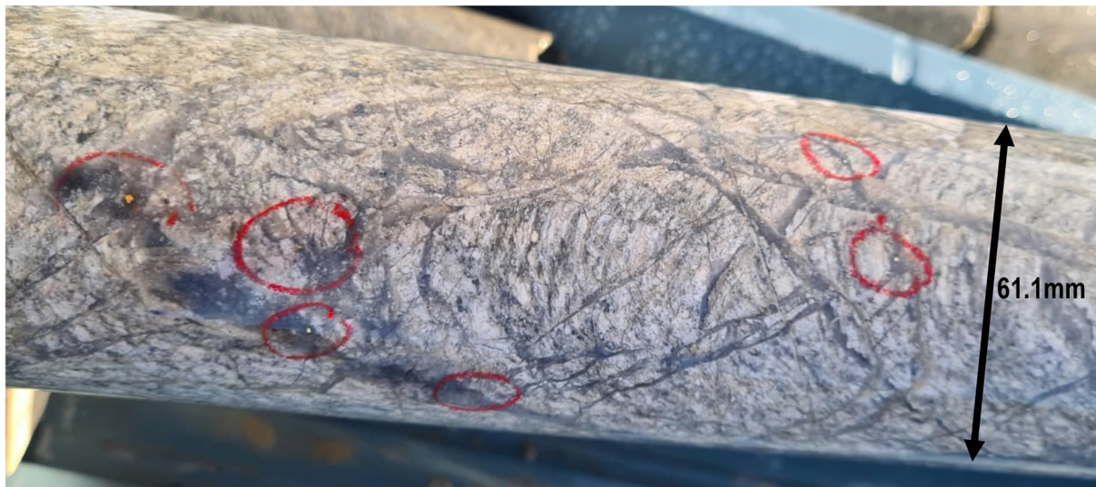
Photo 1. Visible Gold (circled red) in hole 25ENDD001 at 174m down hole. Core diameter is 61.1mm.
