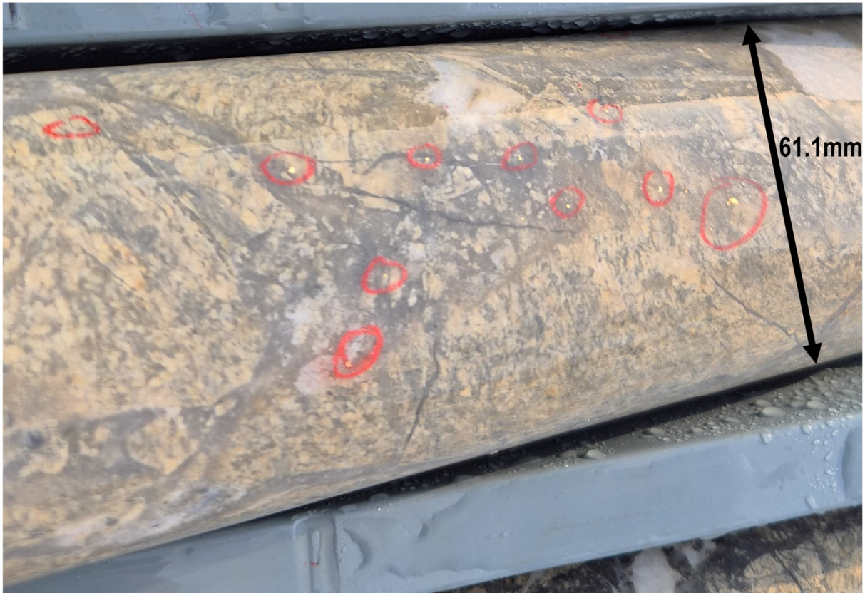
Photo 2. Visible Gold (circled red) in hole 25ENDD001 at 174.5m down hole in quartz veins within granite host rock. Drill core diameter is 61.1mm.
