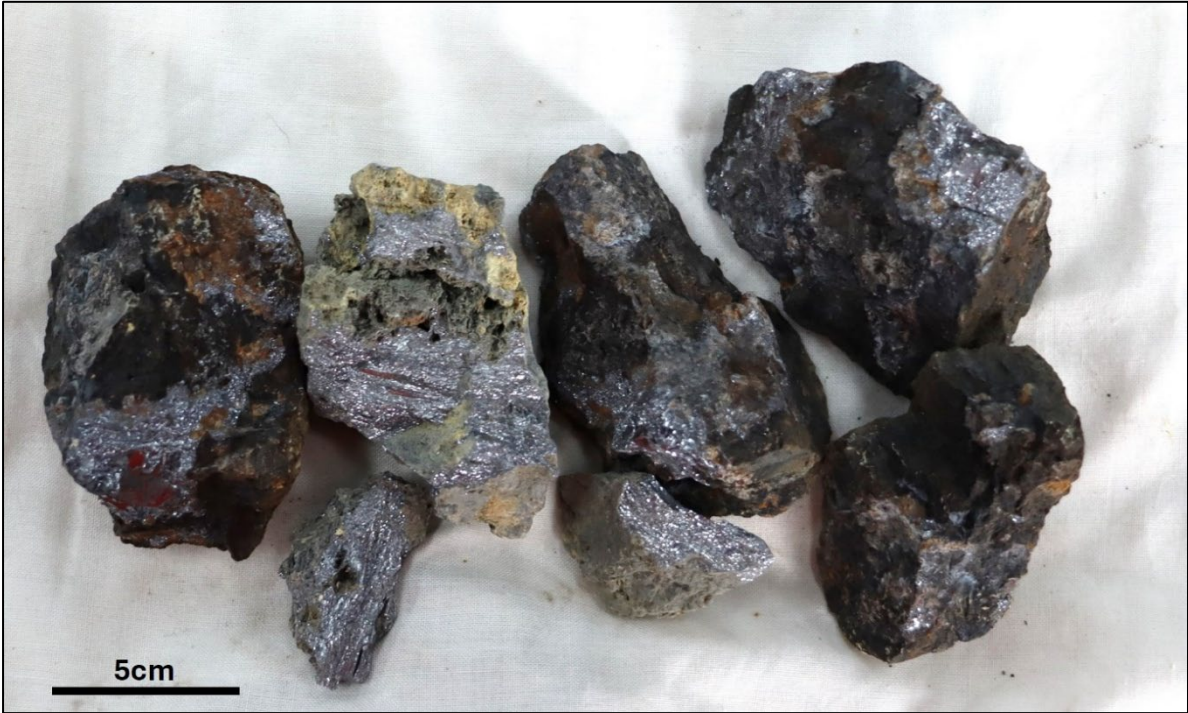
Figure 3 – High-grade silver-bearing galena mineralisation from rock sample AV007 which assayed 1,120g/t Ag with 52.1% Pb and 3.1% Zn
