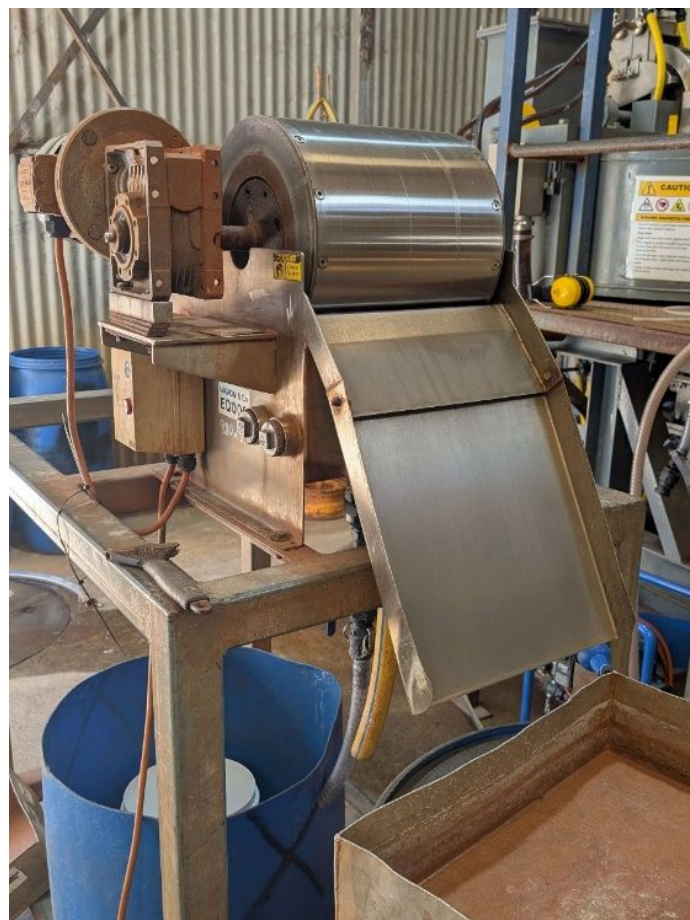
Plate 1: Low Intensity Magnetic Separation (LIMS); NAGROM Laboratories.
