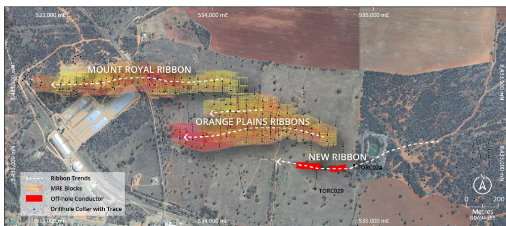
Figure 1: Mount Royal – Orange Plains Prospect – TORC024 & TORC029 off-hole conductor plates and Mineral Resource Blocks > 2,000ppm Copper on aerial photography
