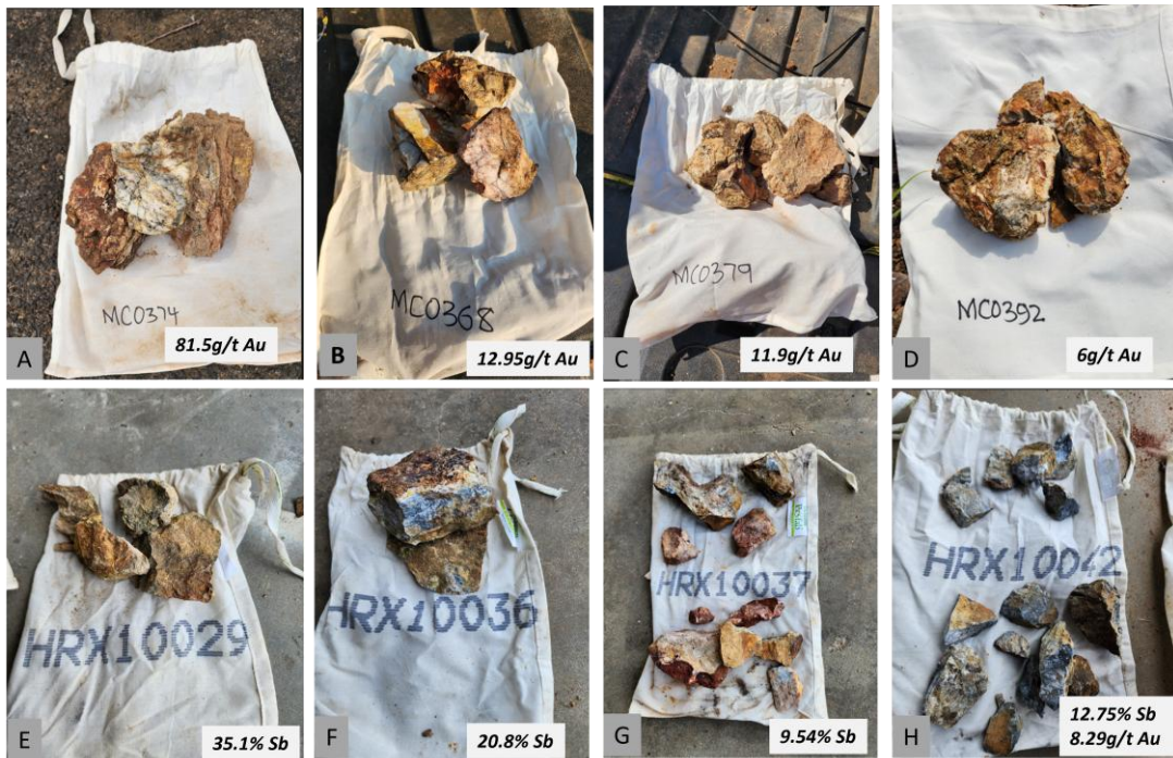
Figure 5: Photo collage for selected samples showing A: MC0374 with 81.5g/t Au, 11g/t Ag, 9840ppm As, 3870ppm Pb, 1275ppm Sb, and 568ppm Zn; B: MC0368 with 12.95g/t Au and 1g/t Ag; C: MC0379 with 11.9g/t Au, 3g/t Ag, and 2890ppm As; D: MC0392 with 6g/t Au, and 3460ppm As; E: HRX10029 with 35.1% Sb, 1.2g/t Au and 4g/t Ag; F: HRX10036 with 20.8% Sb, 0.3g/t Au and 2.2g/t Ag; G: HRX10037 with 9.54% Sb, 1.8g/t Au and 2.5g/t Ag; and HRX10042 with 12.75% Sb, 8.29g/t Au and 1.73g/t Ag. (ASX: 13 February 2025).
