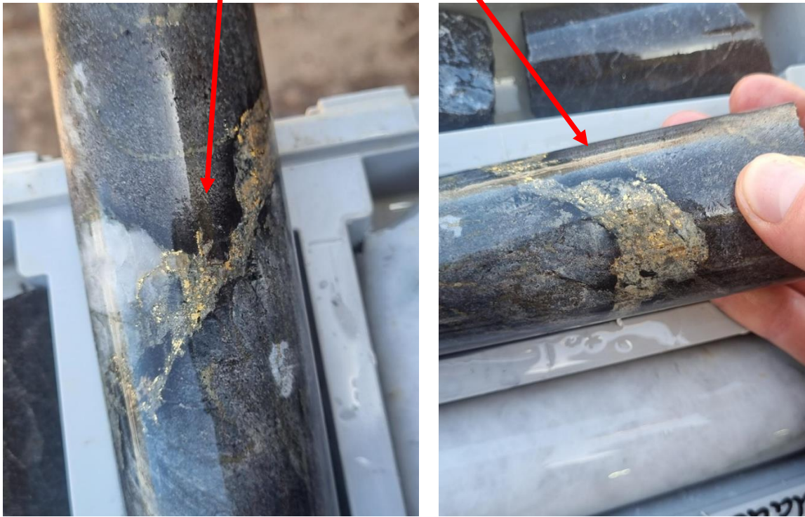
Figure 10 – Hole SKUGGC25032 showing individual assay results and visible gold in core 57.88m.
