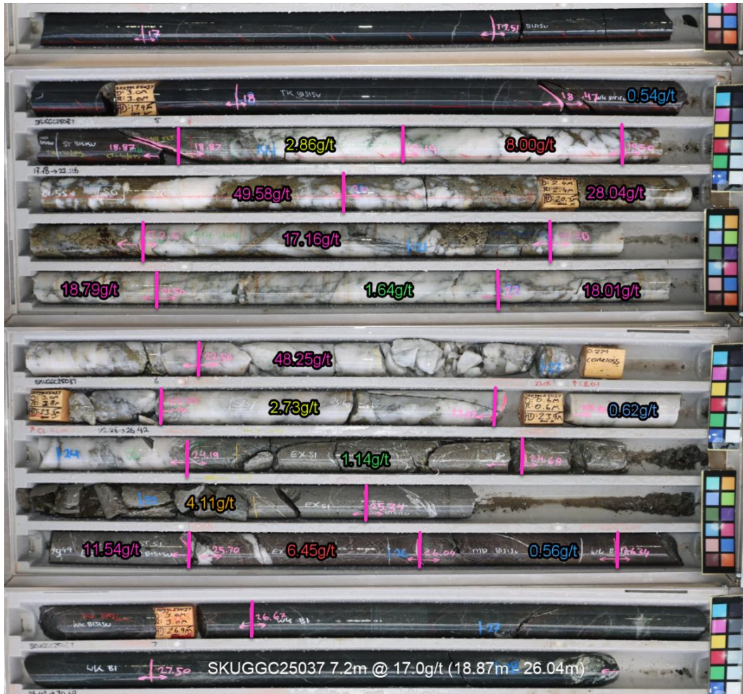
Figure 6 – Hole SKUGGC25037 showing “Blow-out” zone created by the intersection of the D7 lode and Nala Shear. Numbering represents assayed (g/t) gold values for the respective interval..
