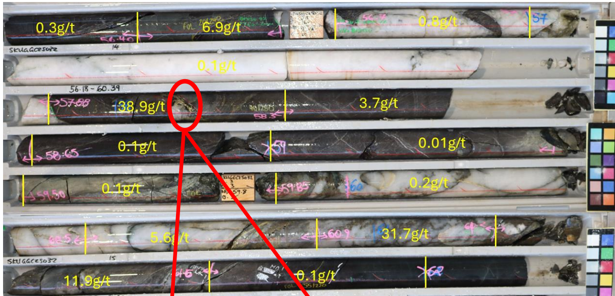
SKUGGC25032 - 5.2m @ 7.1g/t from 56.4m. Numbering represents assayed (g/t) gold values for the respective interval.
