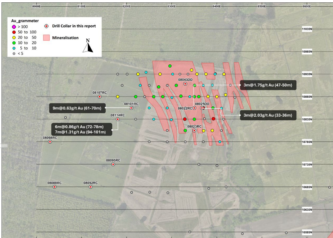
Figure 7: Drill hole locations 15 and gold assay highlights 16 , Northern zone of Chatree South-East Complex.
