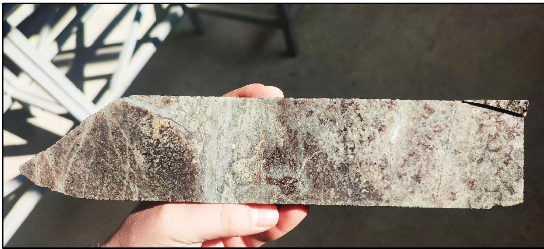
Figure 4. Core photo showing a, b and D veins in a potassic-altered porphyry, from 708m depth in ZRJD24002 (refer to Appendix A for significant intercept details).
