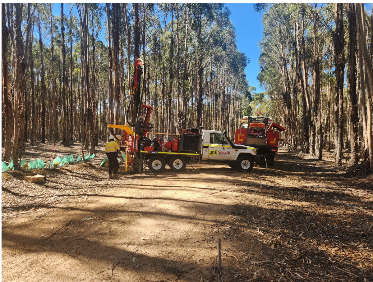
Figure 1. AC drilling underway at the Ivar Prospect, WA
