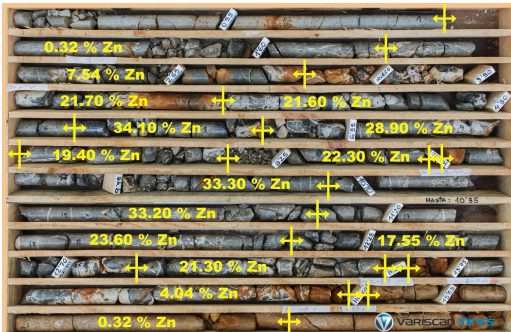
Figure 2. Diamond Drill Core from NDDT059 (15.3m @ 17.42% Zn, 4.40%) illustrating massive sphalerite hosted in dolostone. Hole depth shown is from 0.00m to 16.95m
