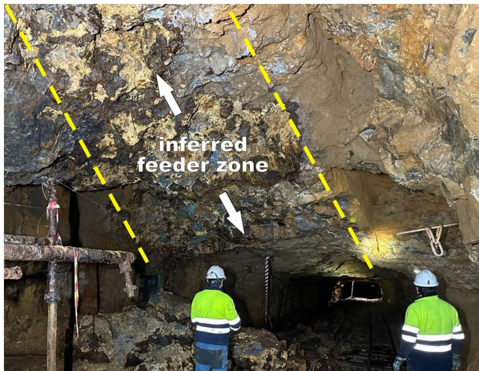
Figure 3. Feeder zone with conspicuous, abundant iron sulphides (partly oxidized on surface) that accompany high-grade zinc and lead sulphide mineralisation
