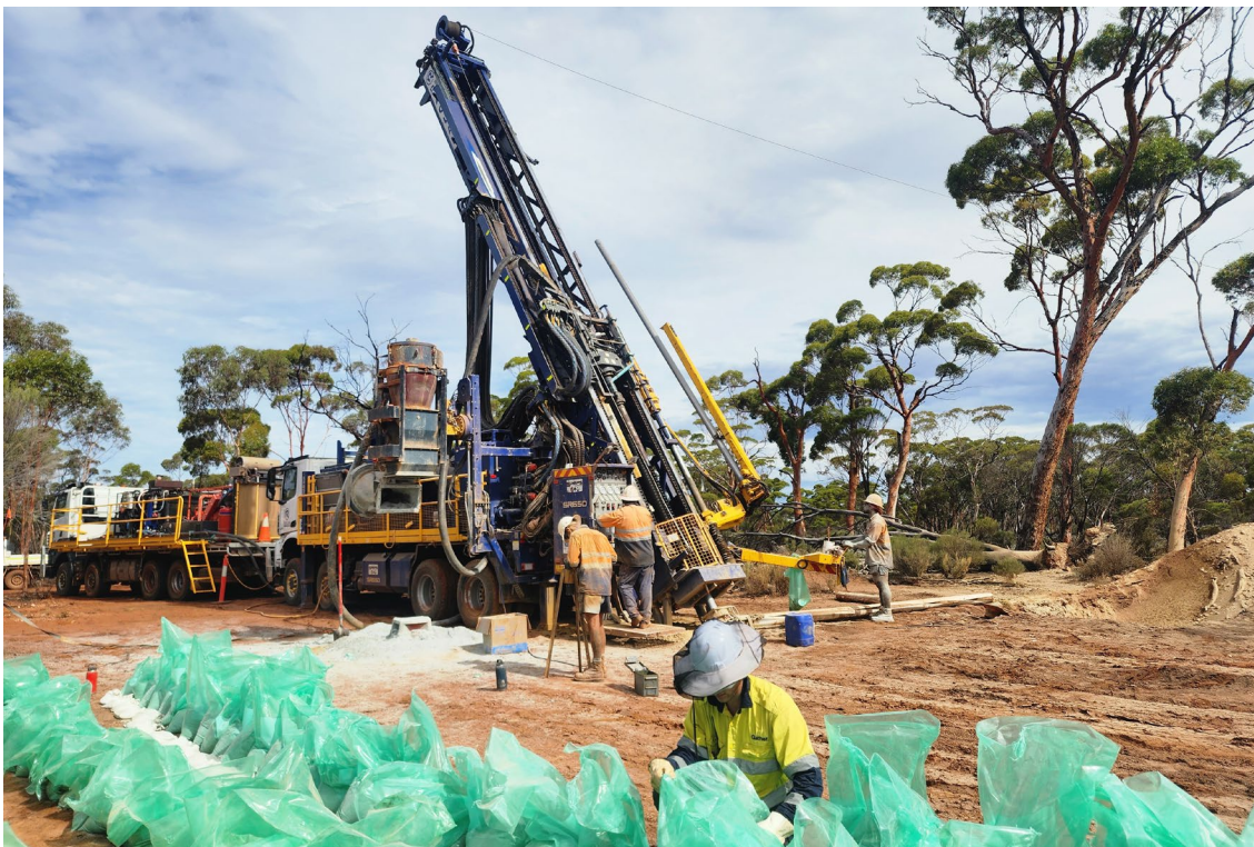
Figure 1. Reverse Circulation drilling at Cognac West prospect, March 2025
