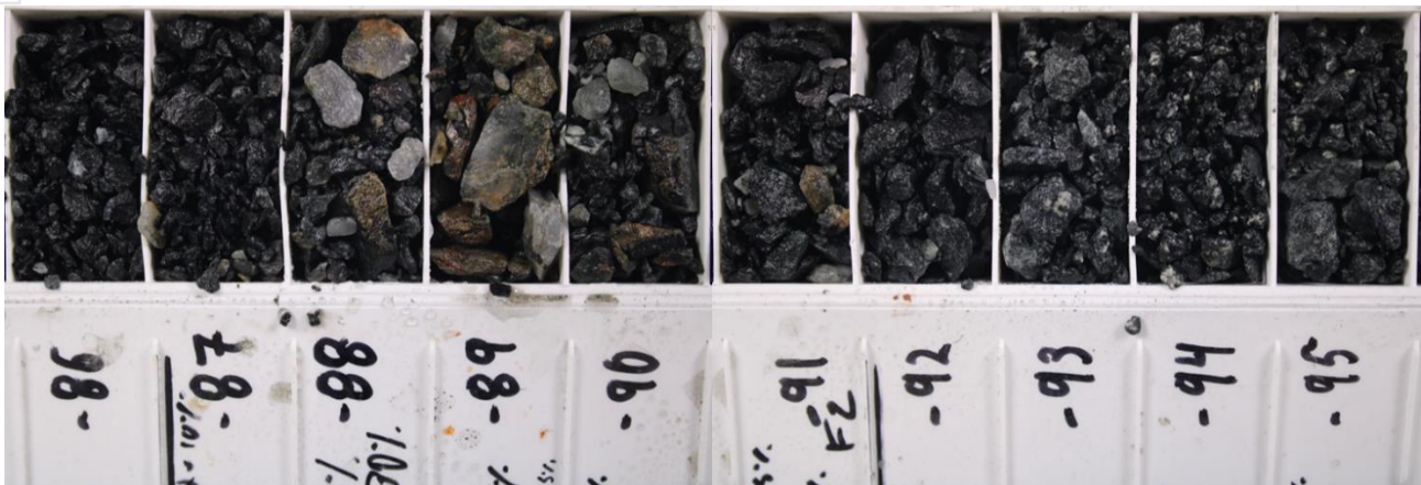
Figure 2 RC chips from mineralised zone in 24PRC141, 4m @ 4.04 g/t from 87m, vertical depth 66.6m. Note abundant sulphides and quartz veins similar in nature of the high-grade gold mineralised zone of the western lode of Paris.
