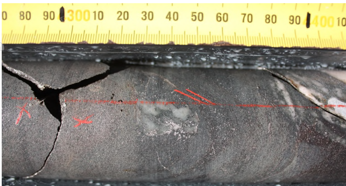
Figure 6. RD045 406.2 – 406.3. fine grained arsenopyrite intergrowth around silica within disseminated pyrrhotite groundmass.
