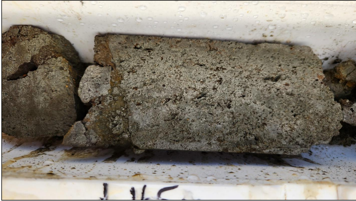
MLJDD018_164.5m_Massive pyrite in Breccia
