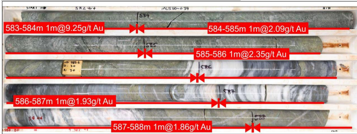
MLJDD039 Silicified ultramafic with fuchsite Alteration
