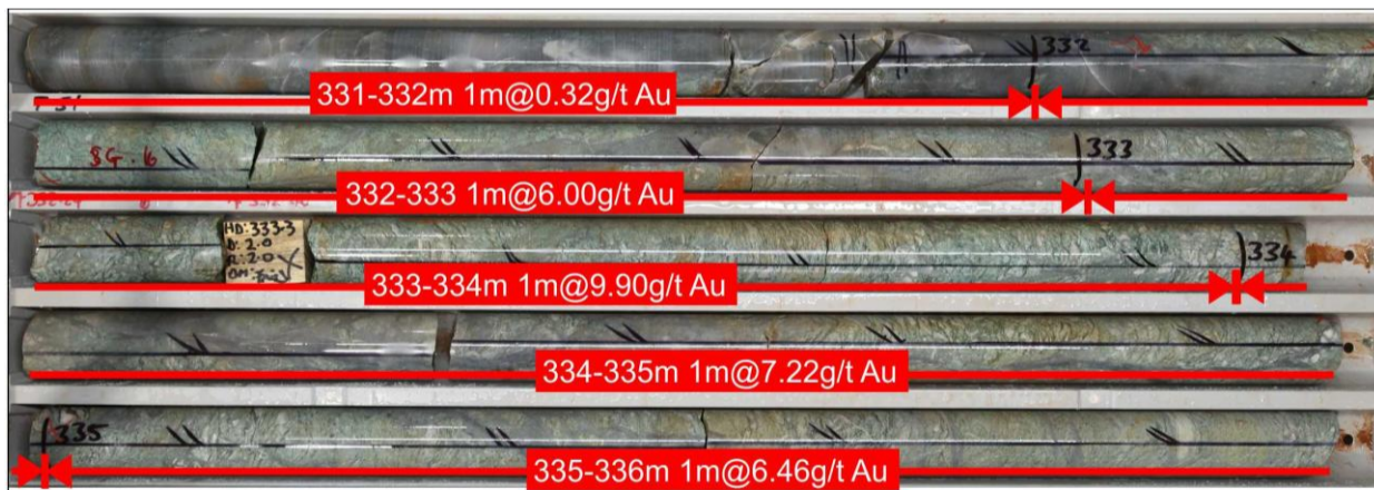
MLJDD042 Silicified ultramafic with fuchsite Alteration
