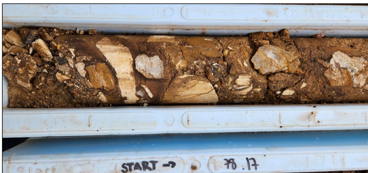
MLJDD020_178.0m_Polymictic Breccia with silica-pyrite clast
