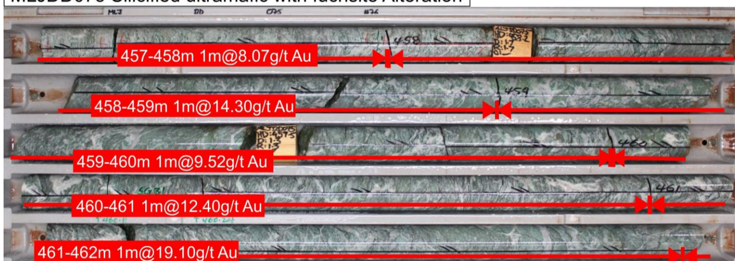
MLJDD075 Silicified ultramafic with fuchsite Alteration
