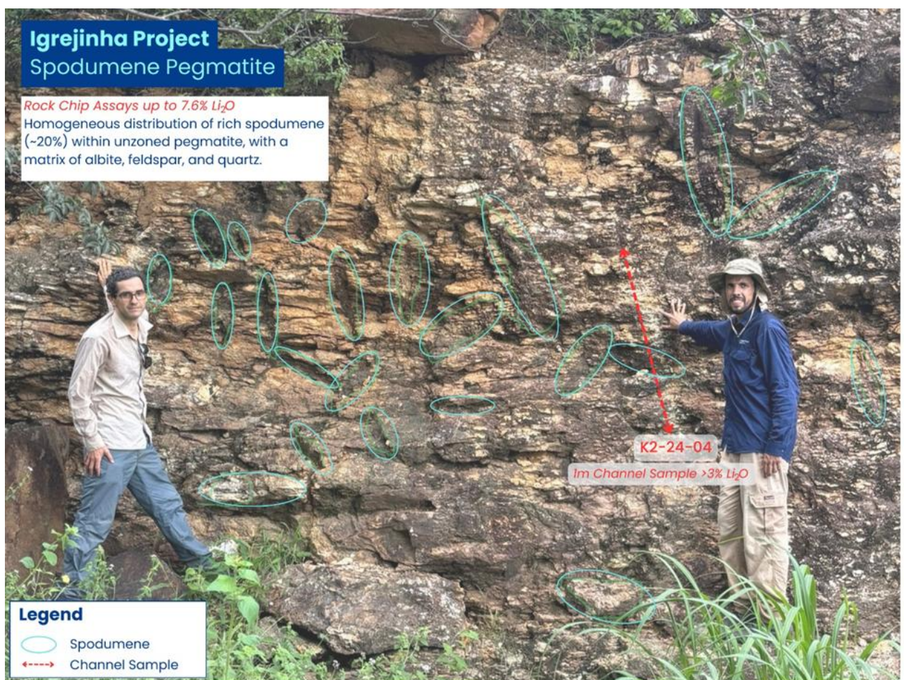
Figure 3 – PEC Team standing in front of outcropping spodumene-bearing pegmatite with individual spodumene crystals up to 50cm in size location of channel sample K2-24-04, located at artisanal workings at the Igrejinha License (830851/2010) 5
