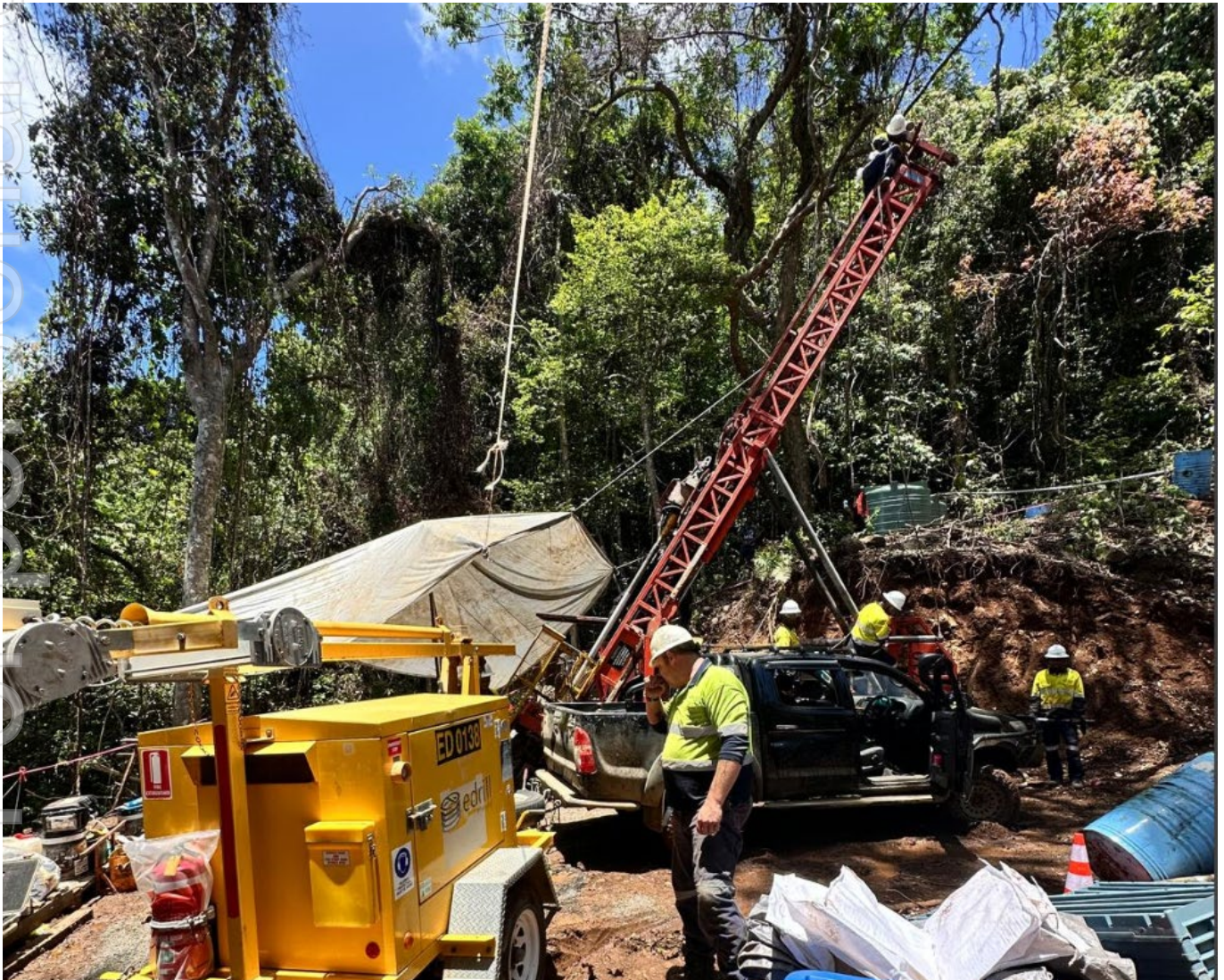
Figure 4 – Diamond drilling at Viani
