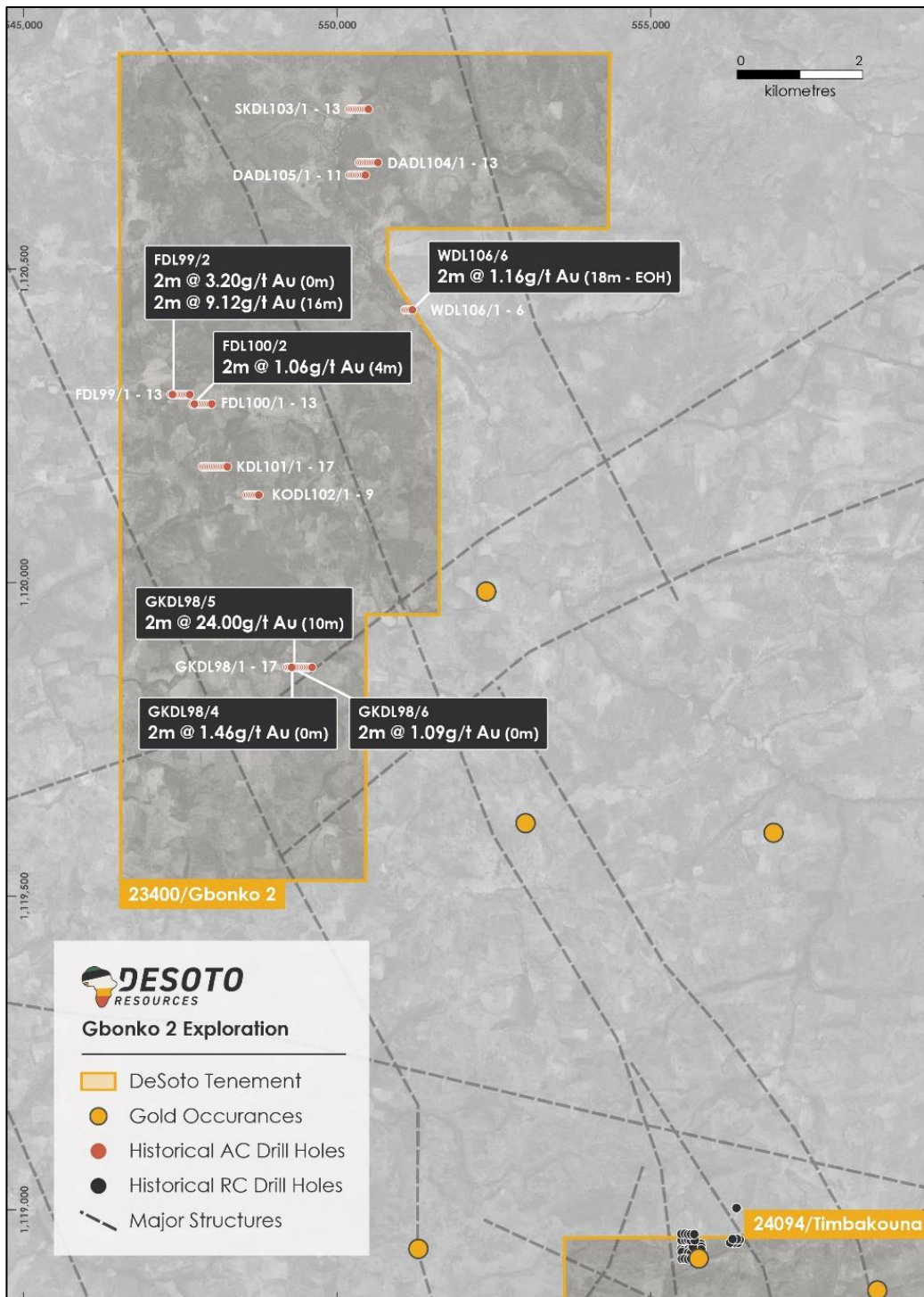
Figure 4 – Gbonko 2 permit showing the location of historical drill holes and significant drill results (>1.0 g/t Au over 2m), known gold occurrences and significant structures.
