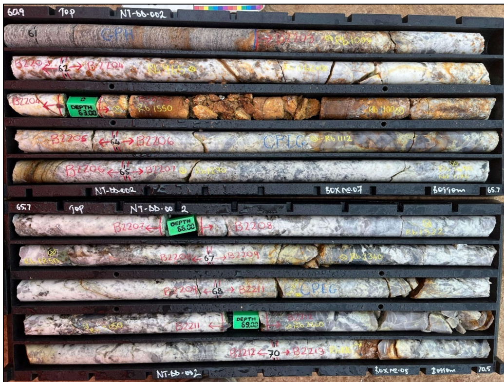
Figure 1: Photo of marked-up core from hole NT-DD-002 from 60.9m to 70.5m. Photo shows mostly coarse-grained pegmatite (CPEG) comprised of principally quartz, feldspar, and mica which intruded into the phyllite (GPH) host rock which can be seen on the top left of the photo. XRF spot readings are marked in yellow on the core where relevant.
