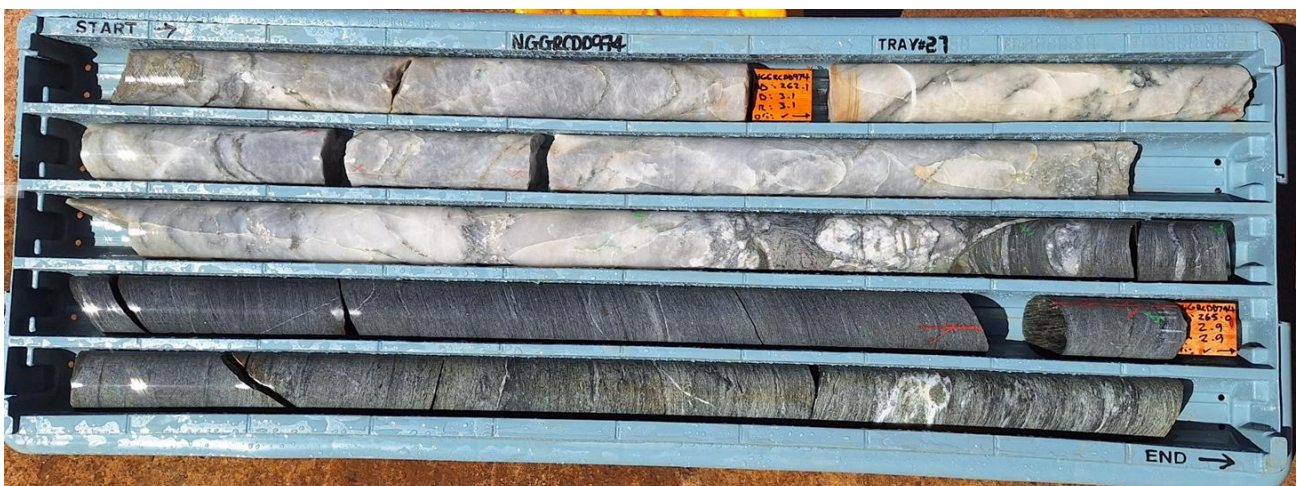
Tray 27 (261.66m – 265.97m) – large quartz-carbonate vein. Sheared and bleached mafic. Footwall to structure at approximately at 263.8m
