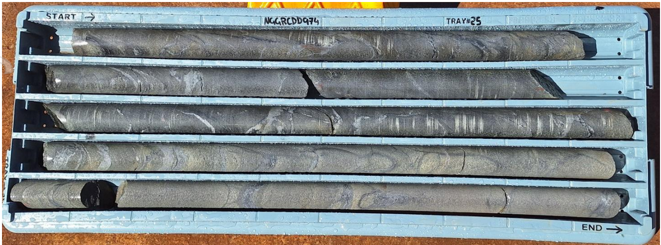
Tray 25 (253.11m – 257.51m) - Sheared and bleached mafic, quartz carbonate veins.
