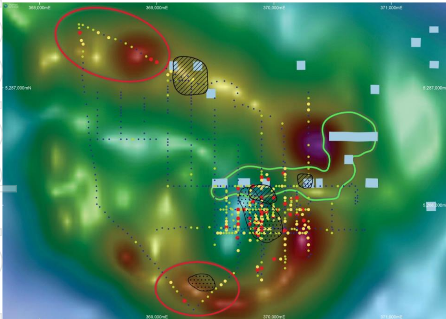
Figure 17: Thomas Creek magnetic annular feature with IP anomaly (green), soils sampling other IP resistivity and chargeability targets shown (see Figure 39 for legend)
