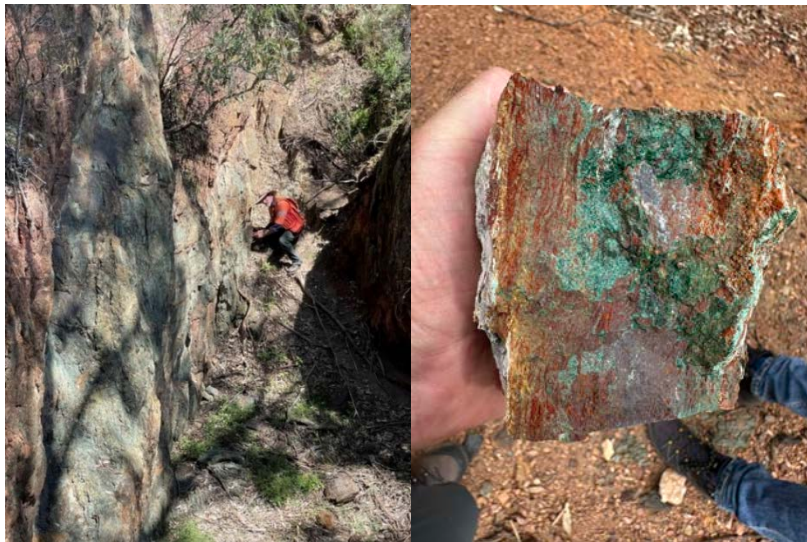
Figure 6. View looking north into the open cut workings at the Mt Everest mine (LHS); Brochantite-malachite bearing massive haematitic gossan 2 from the historic Mt Everest mine (RHS)
