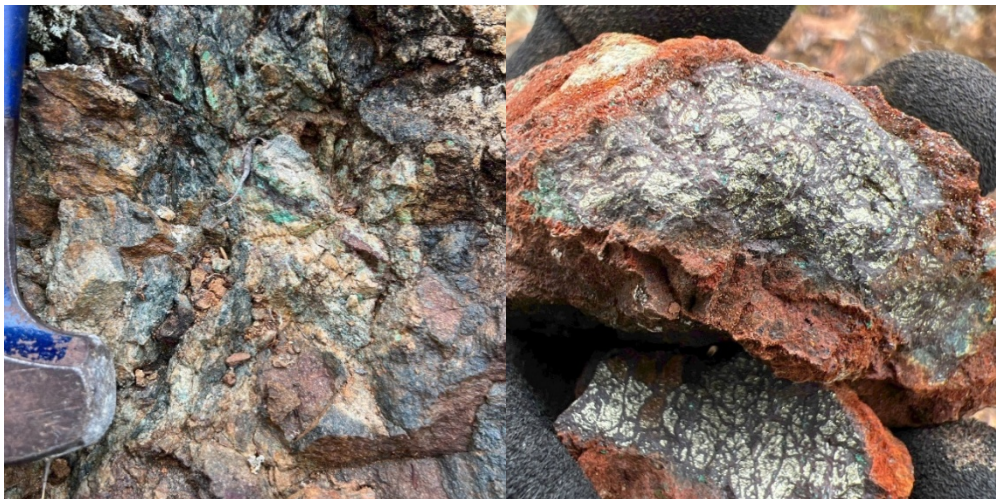
Figure 10. Malachite in sheared ultramafic outcrop (LHS); 10cm wide vein with secondary chalcocite (dark halos) and relic primary chalcocopyrite (RHS) – Back Barb 5
