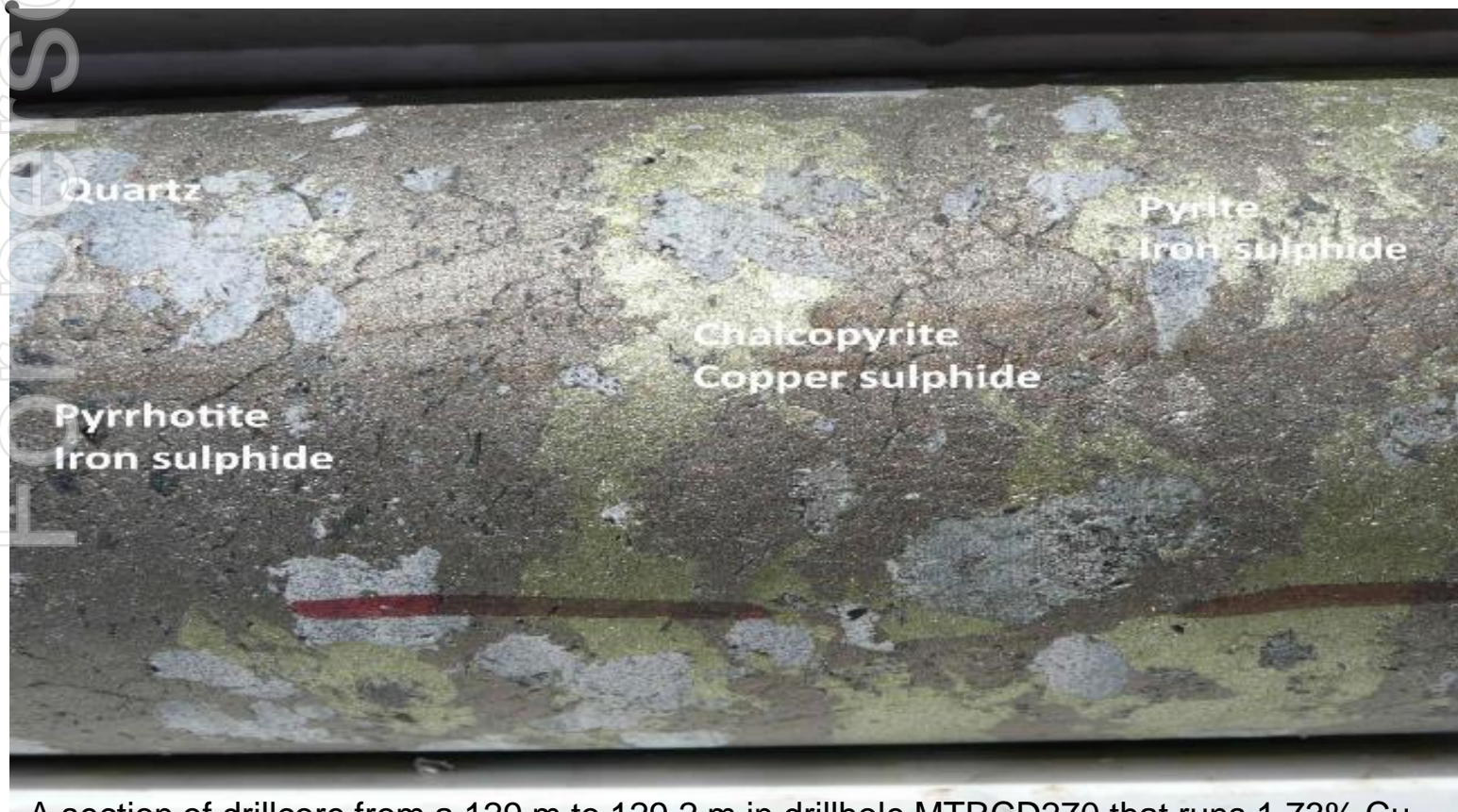
A section of drillcore from a 129 m to 129.2 m in drillhole MTRCD270 that runs 1.73% Cu, 0.17% Co and 0.27 g/t Au ( ASX announcement 27 November 2024 )
