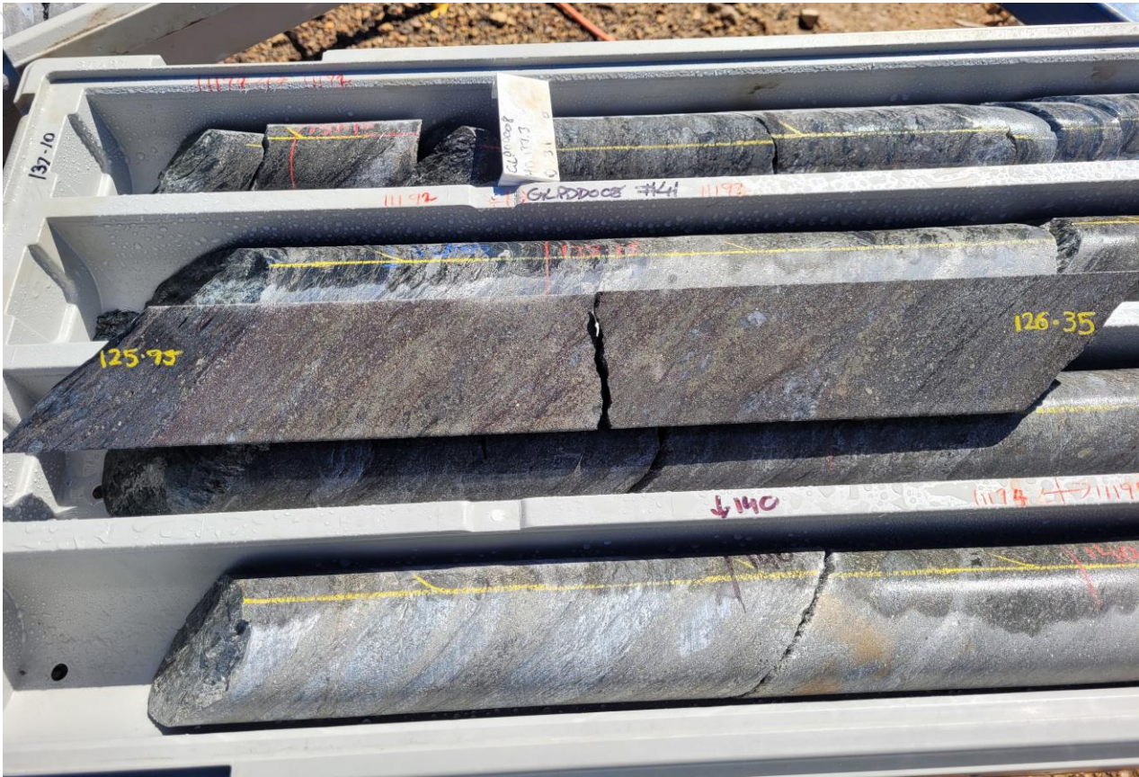
Figure 3: Photo of diamond drill core from GLPDD008 (125.95-126.35m) showing massive to semi-massive sulphide lode with banded pyrite (yellow), sphalerite (red), galena and chalcopyrite. The associated sample interval GRD11176 (126.00-126.55m) returned 9.96g/t AuEq.
