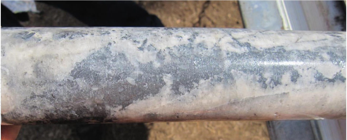
Figure 2 - The Banshee core pictured, drill hole CNDD01 89.9m-90.2m, was part of a zone that assayed 1.25m @ 5.23% Sb and 1.39g/t Au (ASX: GDM Prospectus 2023 and ASX: GDM Sep 2024 ).
