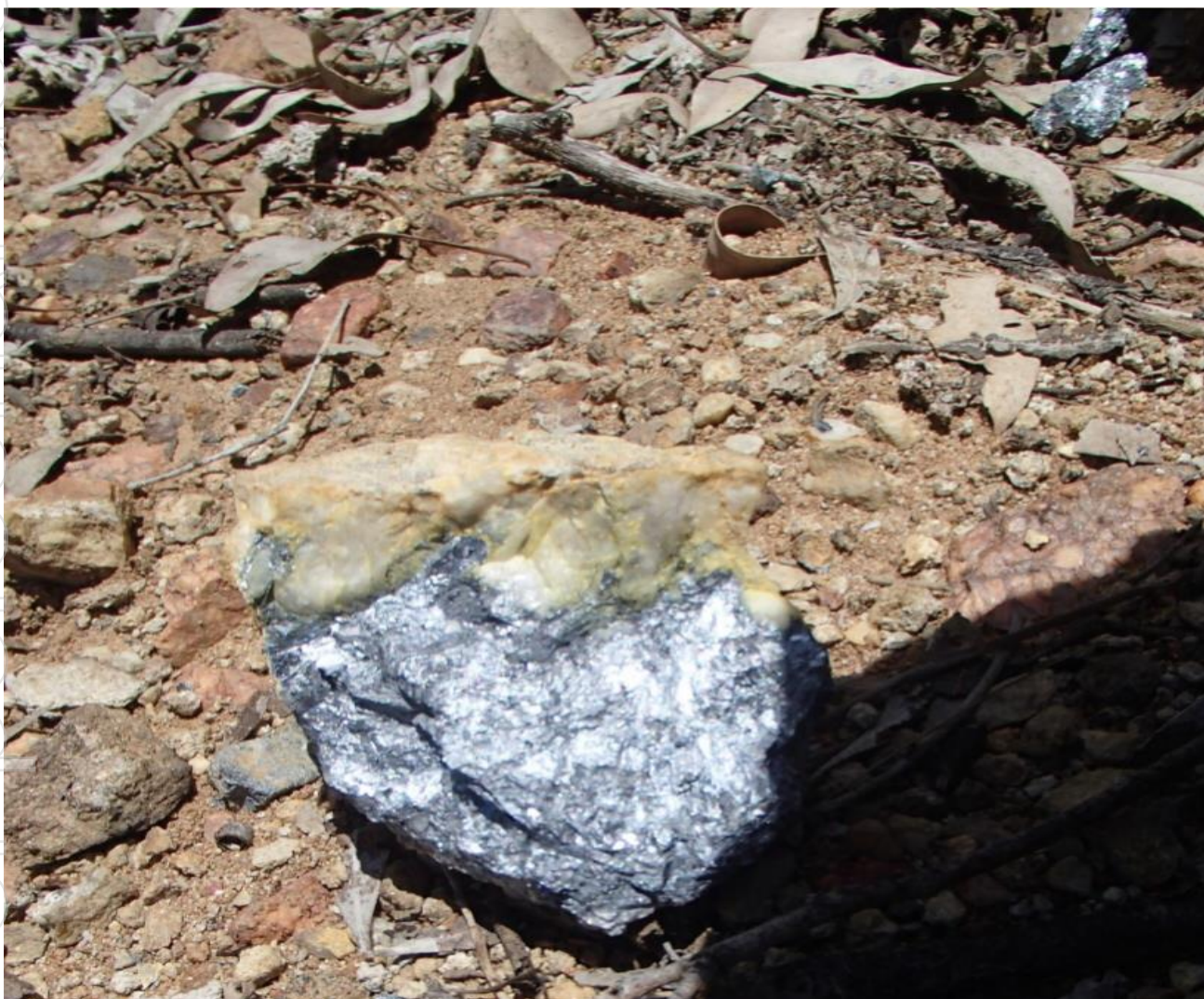
Figure 4 - Banshee mine waste dump material observed by Dart in January 2025 showing antimony mineral (stibnite) with encasing vein quartz
