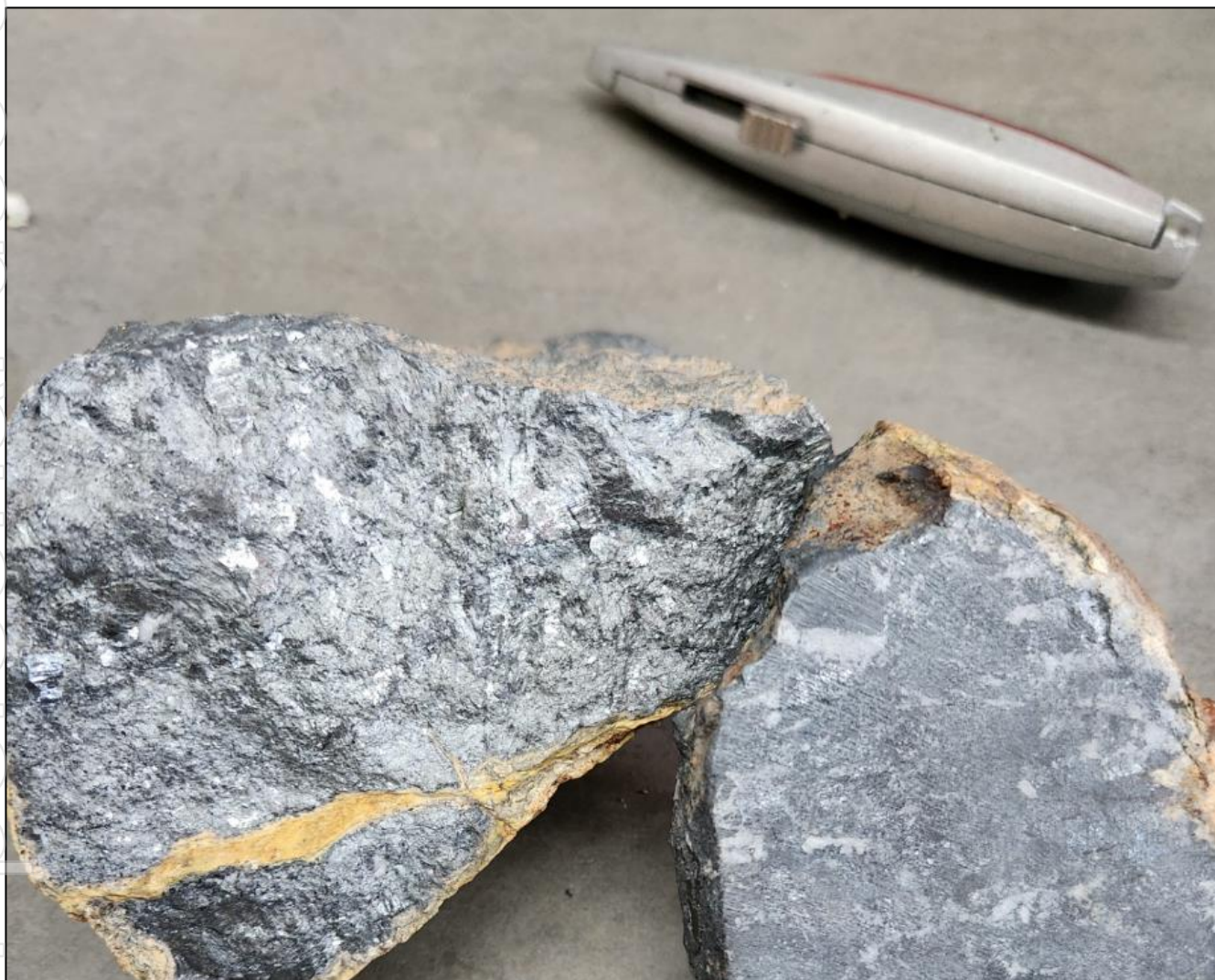
Figure 1 - High-grade stibnite from Banshee antimony mine waste dumps (not In-situ). Broken rock face on the left, sawn rock face on the right. No samples taken or submitted for analysis.
