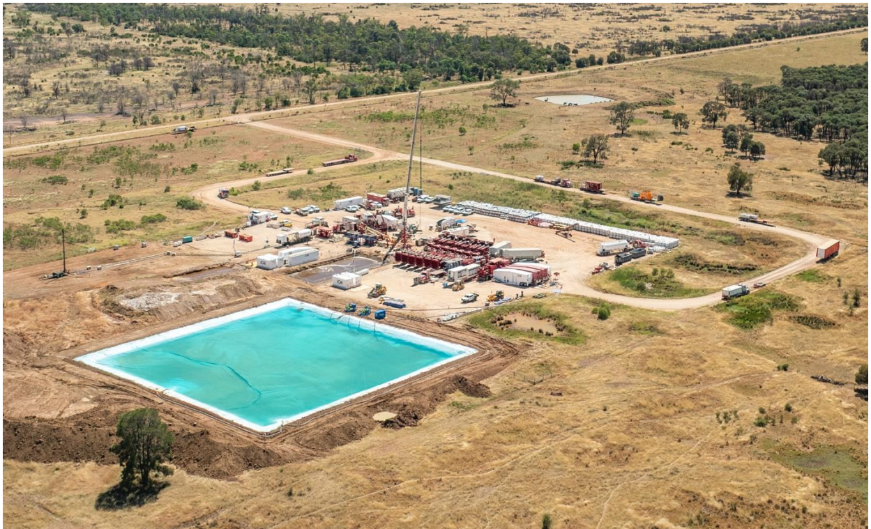
Figure 2: Aerial image of the Canyon-1H fracture stimulation test
