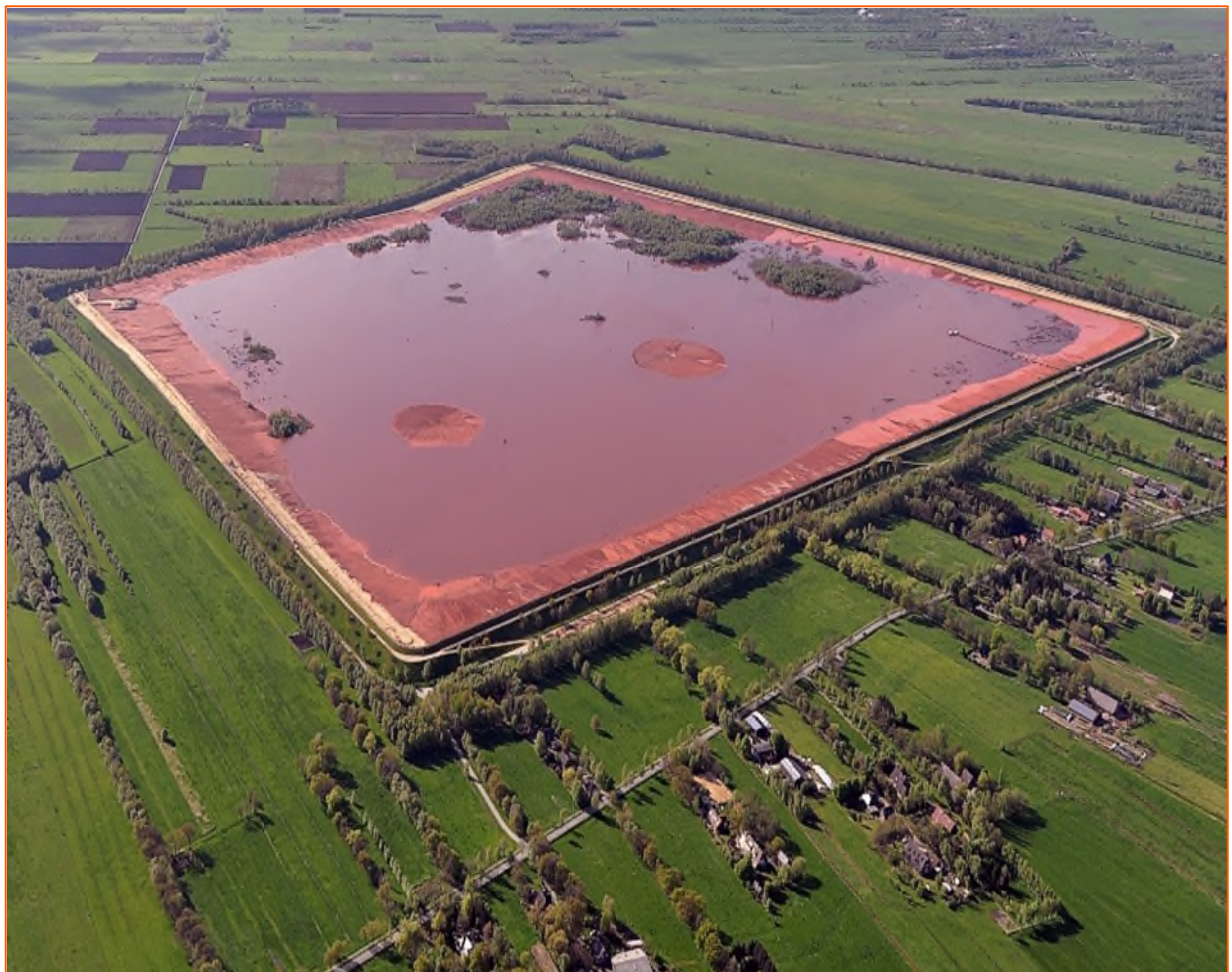
Figure 4: Example of red mud tailings from a bauxite refinery in Germany. Source: Wikipedia .
