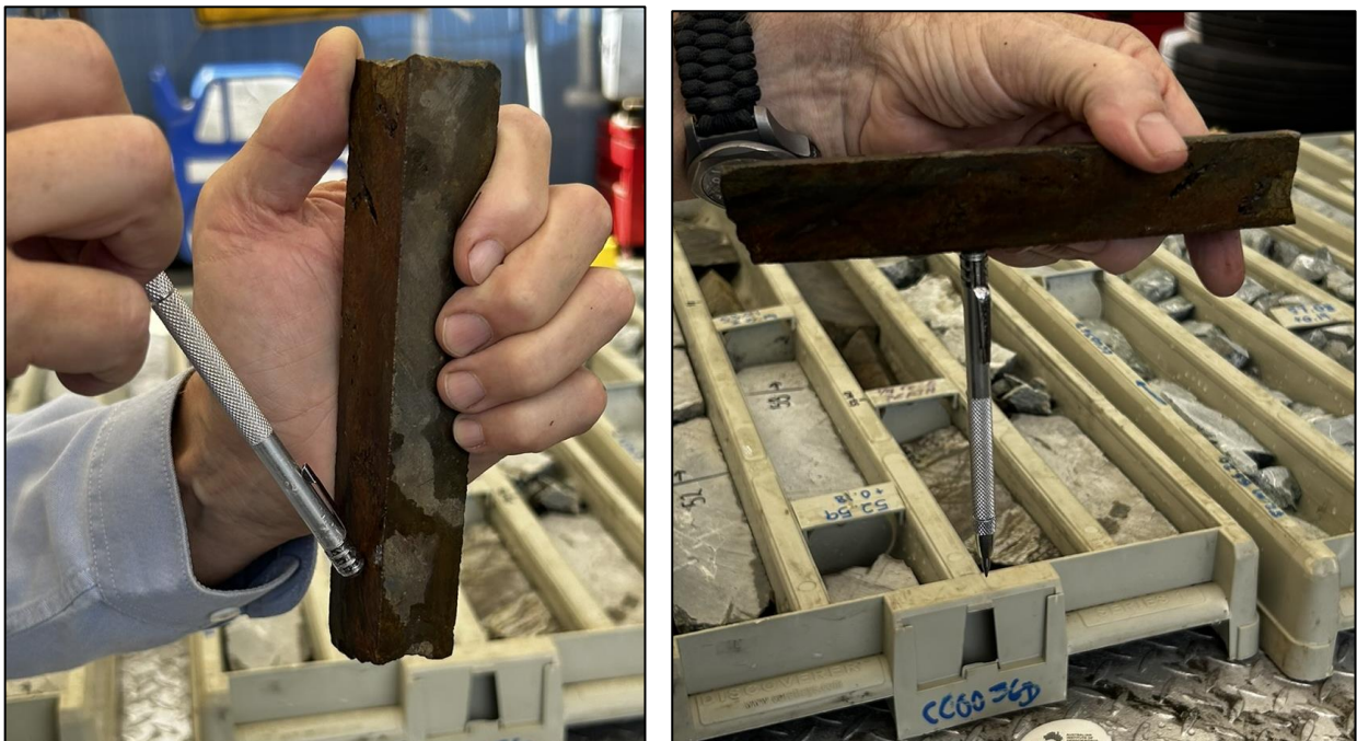
Figure 1: Photos of the highly magnetitic mineralised drill core (pyrrhotite) in diamond core hole CC0036D, responding strongly to a hand-held magnet..
