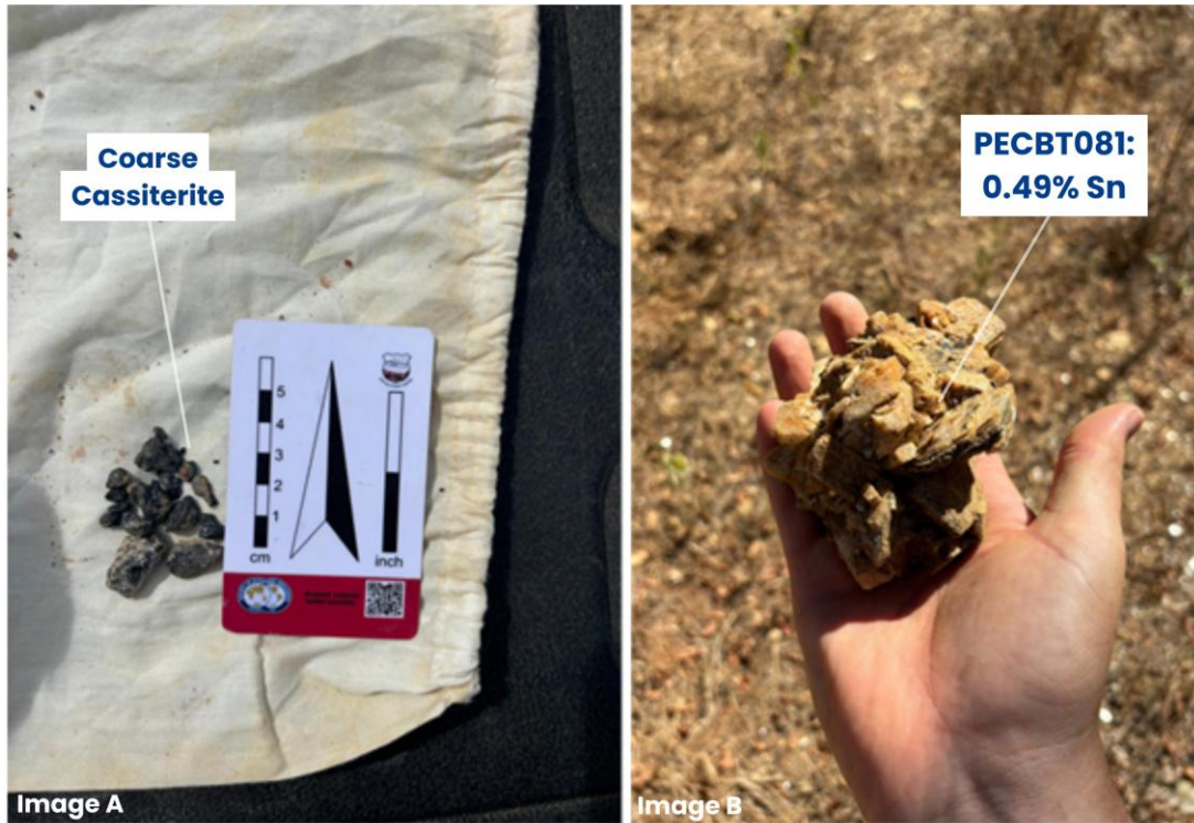
Figure 2: Image A: Coarse Cassiterite. Image B Rock chip with associated Tin assay result at 831542/2004. 7
