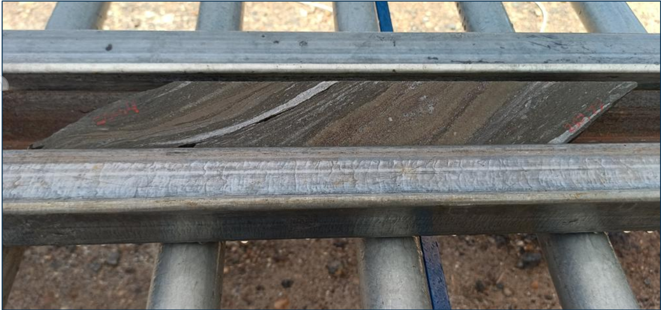
Figure 3: Photo of diamond drill core from GLPDD009 (250.40-250.77m) showing massive to semi-massive sulphide lode with banded pyrite (yellow), sphalerite (red), galena and chalcopyrite. The associated sample interval GRD11404 (250.15-251.15m) returned 5.49g/t AuEq.
