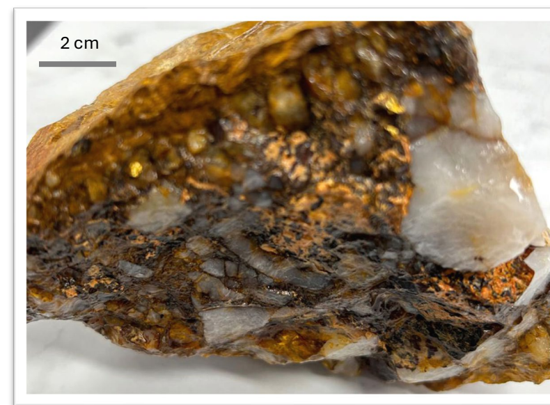
Visible gold in the Revere Reef system, about 12 cm quartz vein outcrop in shallow costean
