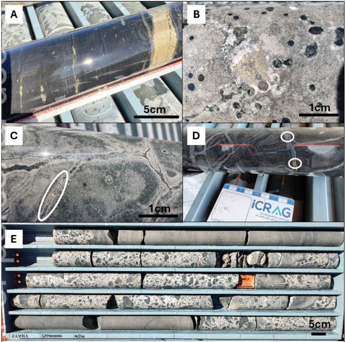
Figure 4: (A) lenses of banded pyrite within interbedded shale-volcaniclastic rocks, considered responsible for the conductive response (835m); (B) Chalcopyrite (mineralogy confirmed with XRF) with pyrite and quartz-carbonate veining and within the basalt sequence (1,031m); (C) Chalcopyrite within pyrite veining (confirmed with XRF), at 1,026m; (D) Chalcopyrite with quartz-carbonate veining, at 878m; (E) Carbonate matrix breccia with basaltic clasts, with pyrite both disseminated and rimming clasts (918m), potential VHMS feeder?
