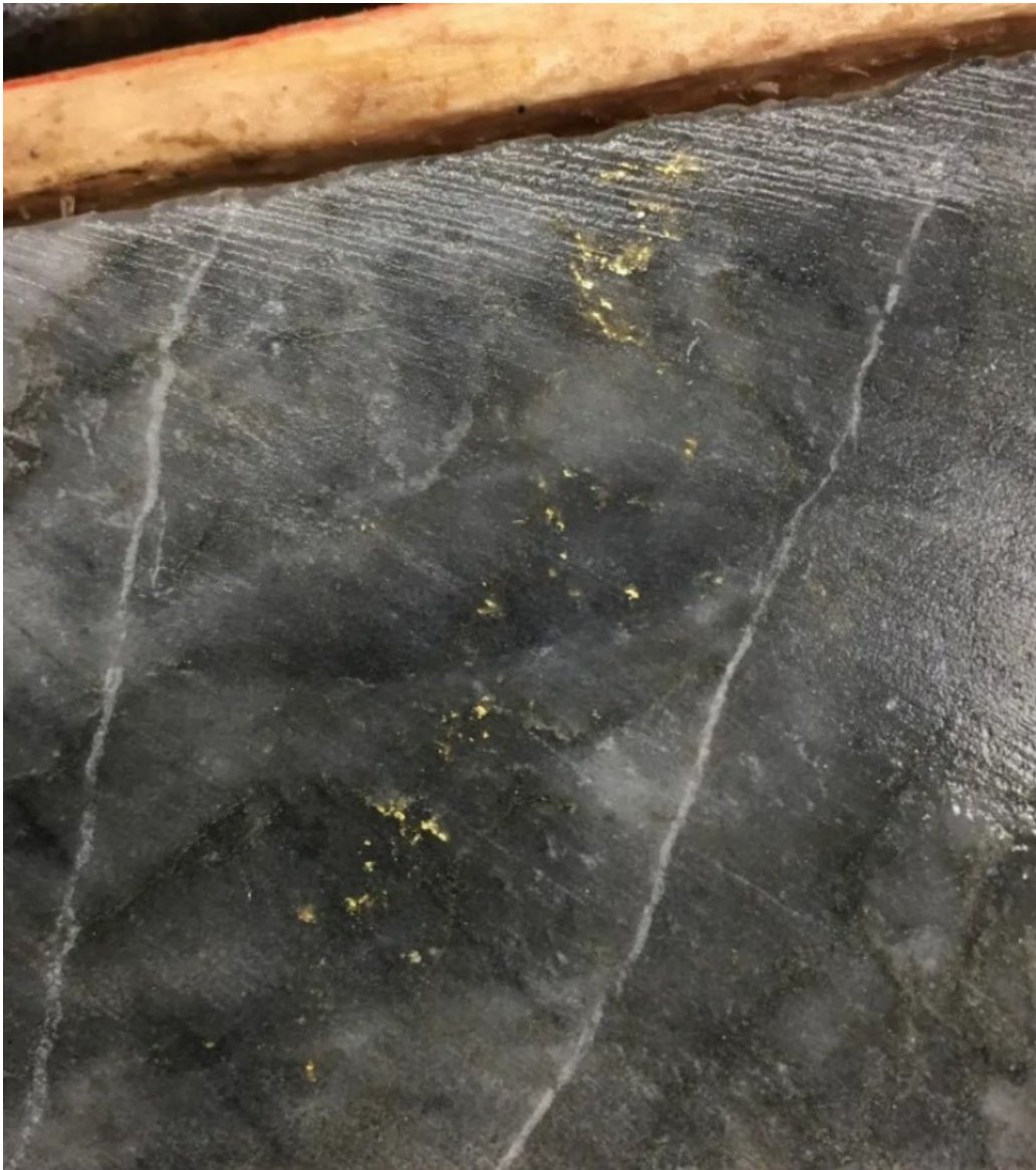
Figure 3: Photo of core from drillhole B0-21-08 at the Paquin East prospect showing Visible Gold within characteristic blue-grey quartz (184.5m). The one metre interval 184-185m assayed 1m@ 129.25g/t Au. This was within 9m @ 16.96g/t Au from 178.5m vii .
