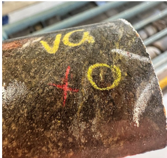
Figure 3: Visible gold at 270m downhole in hole 25KVUG0530 circled in yellow
