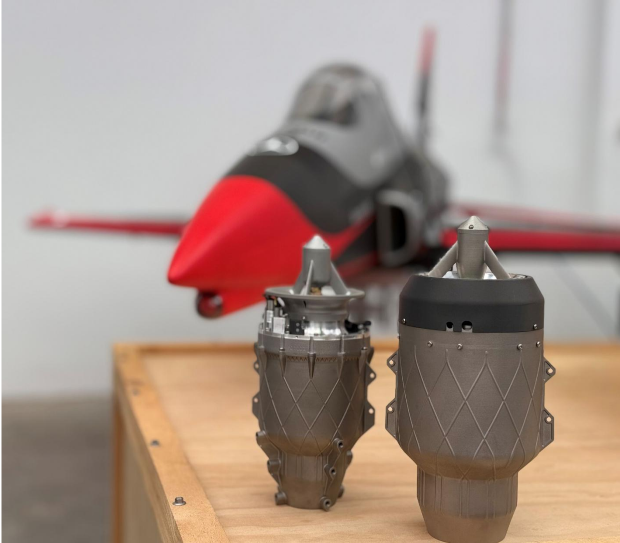
AU4 Micro Gas Turbine, sitting alongside the AU2
