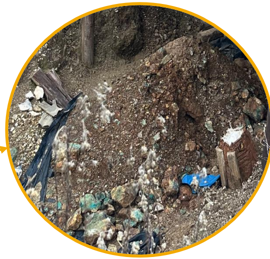
Figure 10: Sample R14 from discovery of previously unknown shaft present at Irka SW Porphyry-Skarn at the base of the 10m pit which has been mined. Inspection of the shaft indicated a depth further depth of ~15m. Mined footwall of shaft can be seen stockpiled at bottom of the image, with significant presence of copper bearing ore, indicating the supergene copper zone extends to a depth of 25m and remains open . Zoom-in of stockpile with visual copper present can be seen circled below.
