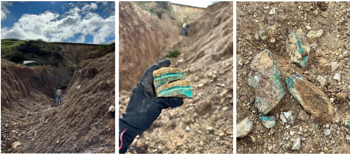
Figure 9: Left – Historic pit at Irka SW Porphyry-Skarn mined to 10m depth being investigated. Middle – Presence of supergene copper mineralisation of Azurite and Malachite at base of pit. Right – Further presence of highly enriched copper bearing ore present at base of pit.
