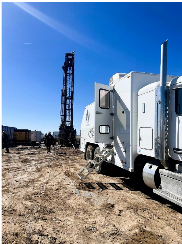
Air drilling the Lyons Sandstone (left) and open-hole logging of the Lyons at TD (right)
