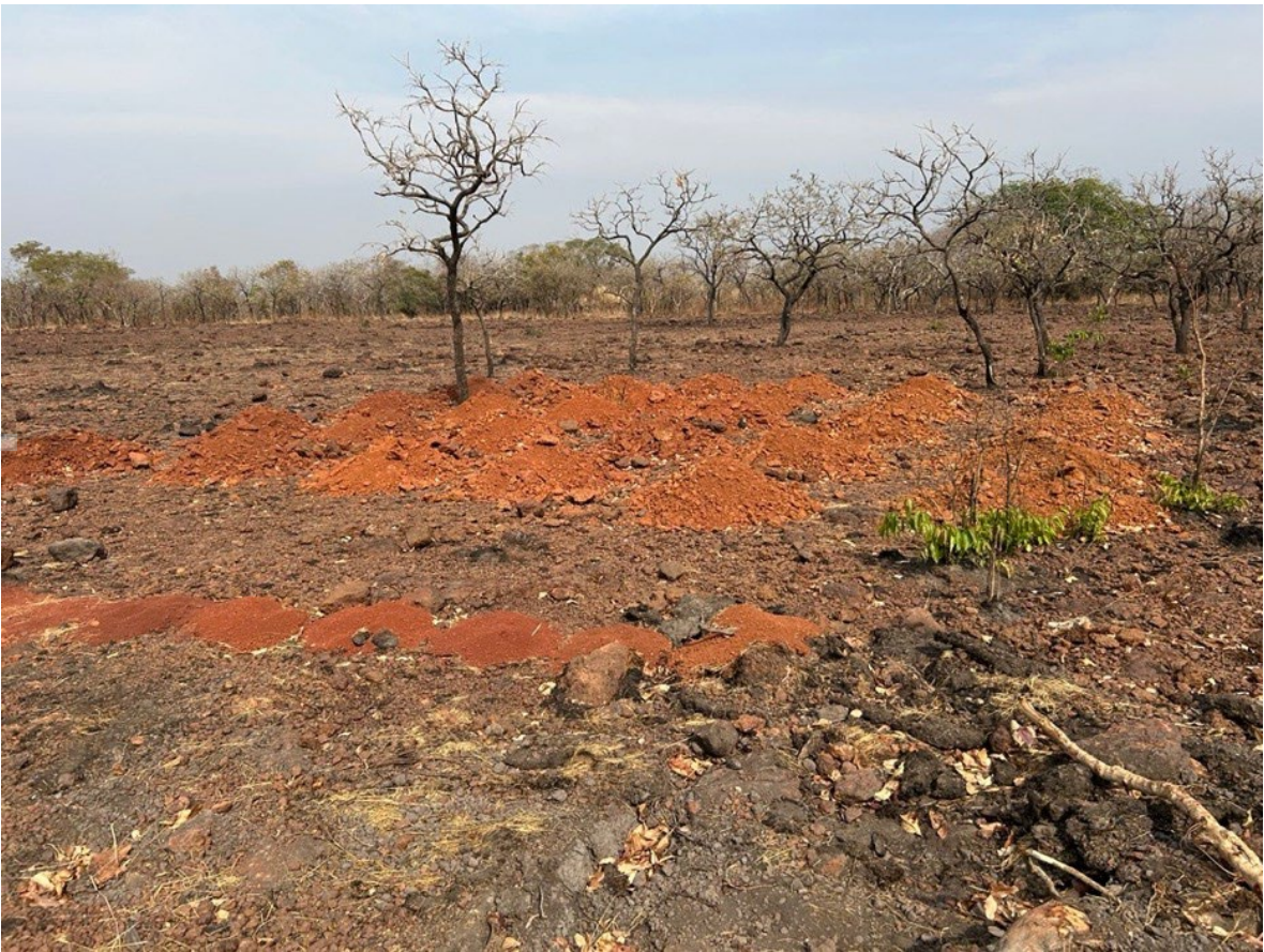
Figure 10. Boussoura North West Auger BS000121, drill cuttings sampled in 1m intervals in foreground, excavated bulk sample pit (BSP006) cuttings at 20cm intervals in background
