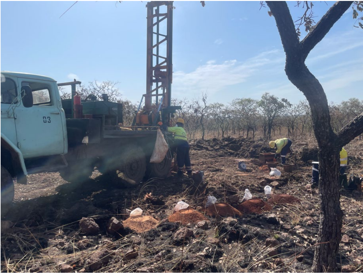
Figure 7. Partially completed auger hole, Central Boussoura Plateau, with logged and sampled drill cuttings noted in foreground
