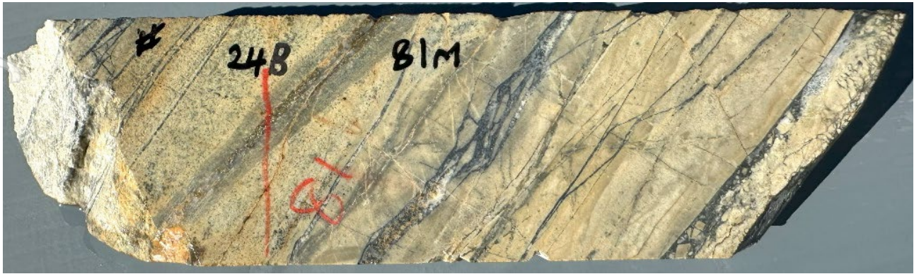
Fig 11. Photo Half HQ Core . Hole 25CAEDD024 at 81m - sericite altered and heavily veined hornfelsed siltstone with prominent sheeted veins of quartz-ankerite-pyrite-molybdenite -minor chalcopryite. -1m interval 81m-82m : 666 ppm Mo, 0.11% Cu, 0.02 g/t Au, 1.3 g/t Ag, 0.5% S.
