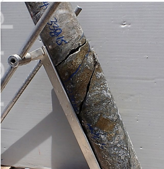
Fig 13. Photo full HQ core Hole #24 ,157.2m, oriented in core oriented frame, hole drilling to west south west , view looking south east , hole at 157m inclined at -68 degrees toward 251 degrees mag: Infill hydrothermal breccia, with slabby/shingle clasts aligned normal to direction of hole. Slab alignment averages dipping 45 degrees, striking 010 degrees mag , dip direction 100 degrees mag. Clasts dominated by light grey,sericite altered hornfels , with infill of carbonate (white) , quartz (colourless), chlorite infill & altered rock flour (green) , pyrite (brassy) . 1m Interval 157m-158m grades 0.53%Cu, 0.13 g/t Au, 8 g/t Ag, 3.09% S.
