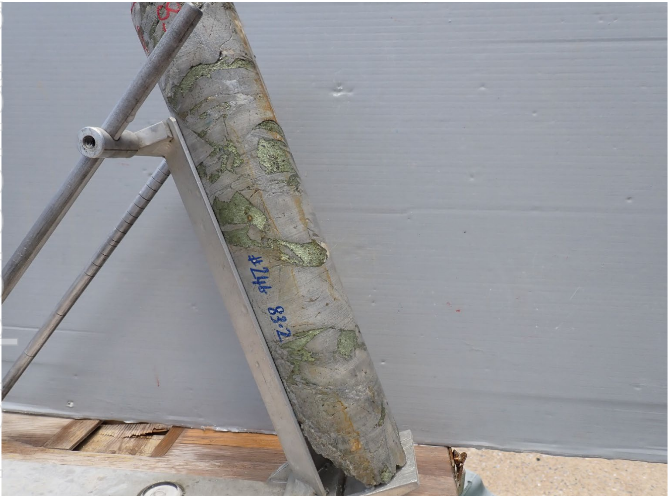
Fig 12. Photo full HQ core Hole #24, oriented in core oriented frame at 83.2m, hole drilling to west south west , view looking south east , hole at 83m inclined at -68 degrees toward 248 degrees mag: Chalcopryite rich Hydrothermal Infill Breccia. Clasts dominated by yellow grey, sericite altered hornfels, with infill of chalcopryite (golden) , pyrite (brassy) ,minor calcite (white) ,quartz (glassy).
