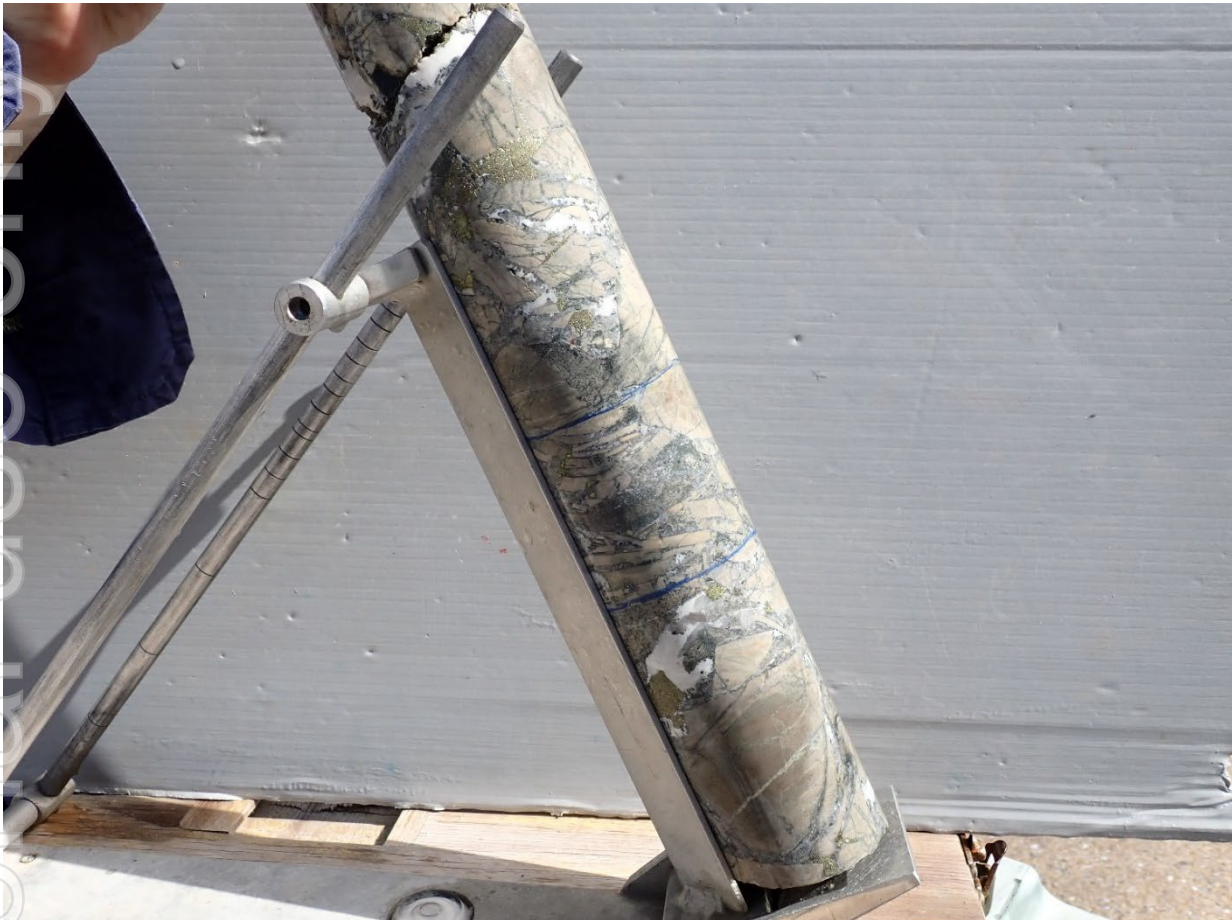
Fig 13. Photo full HQ core Hole #24 ,157.2m, oriented in core oriented frame, hole drilling to west south west , view looking south east , hole at 157m inclined at -68 degrees toward 251 degrees mag: Infill hydrothermal breccia, with slabby/shingle clasts aligned normal to direction of hole. Slab alignment averages dipping 45 degrees, striking 010 degrees mag , dip direction 100 degrees mag. Clasts dominated by light grey,sericite altered hornfels , with infill of carbonate (white) , quartz (colourless), chlorite infill & altered rock flour (green) , pyrite (brassy) . 1m Interval 157m-158m grades 0.53%Cu, 0.13 g/t Au, 8 g/t Ag, 3.09% S.
